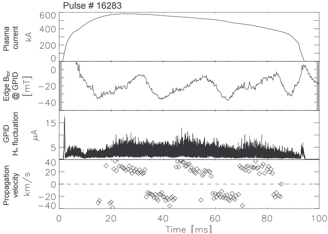
Fig 1: time evolution of the plasma current, toroidal magnetic field at GPID location,  $H_\alpha$  emission intensity and propagation velocity of fluctuations from GPID measurements
