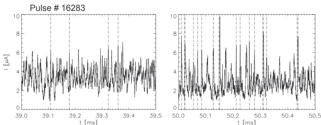
Fig. 5: signal samples of  $H_{\alpha}$  emission, with “intermittent” events identified at  $2 \mu s$  scale.
