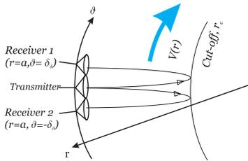
Figure 1 Poloidal correlation reflectometry experimental scheme
