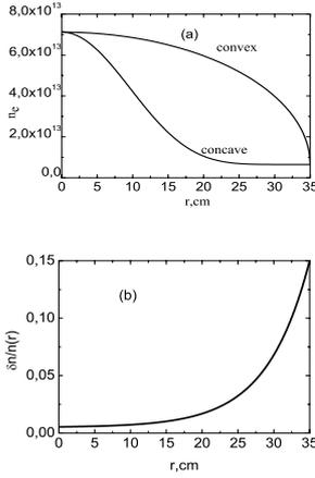
Figure 2 (a) background density profiles (convex and concave); (b) density fluctuation level profile
