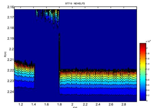
**Figure 5: He beam measurement of the density at the plasma edge. The limiter of the antenna is located at R=2.23m.**
