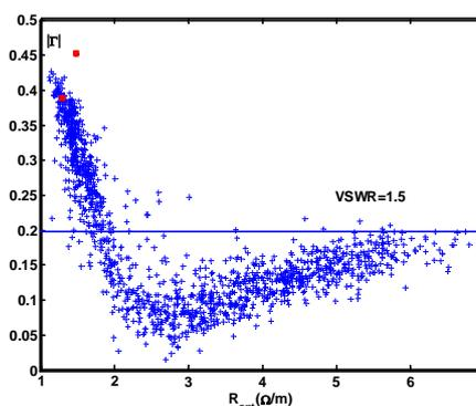
**Figure 7 Reflection coefficient at the generator as function of antenna loading resistance**
