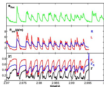
**Figure 6 Recycling flux, antenna loading resistance and reflection coefficient as function of time**
