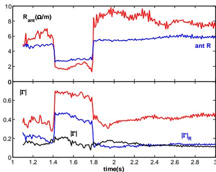
**Figure 4: Evolution of antenna loading resistance and of the reflection as function of time. At t=1.4s the plasma is suddenly displaced away from the antenna.**
