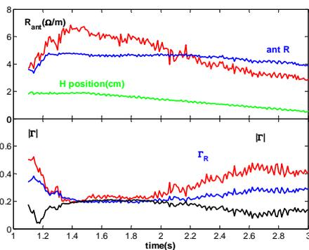
**Figure 3: Evolution of the antenna resistance and of the reflection coefficient during a slow displacement of the plasma away from the antenna**
