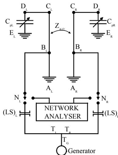
**Figure 1: Equivalent circuit of the antenna**
