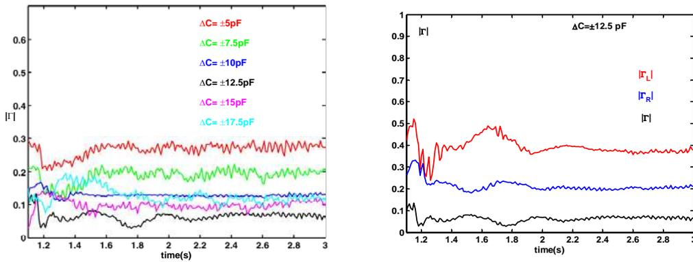
**Figure 2: Reflection coefficient  $|\Gamma|$ ,  $|\Gamma_L|$  and  $|\Gamma_R|$ , in the respective sections generator- $T_G$ ,  $T_L-B_L$  and  $T_R-B_R$  for the given values of the detuning  $\Delta C_p$**
