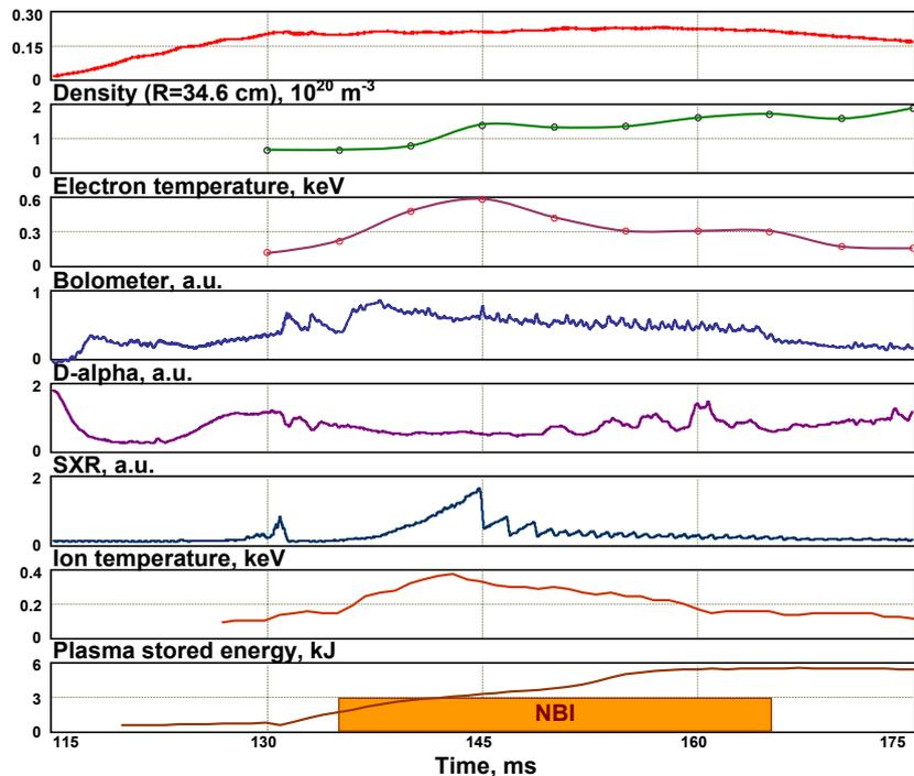
FIGURE 5. Time evolution of plasma parameters in shot #13731.  $P_{NB} = 0.55$  MW,  $E_{NB} = 28$  keV
