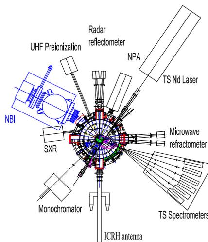
FIGURE 1. NBI layout on Globus-M.
