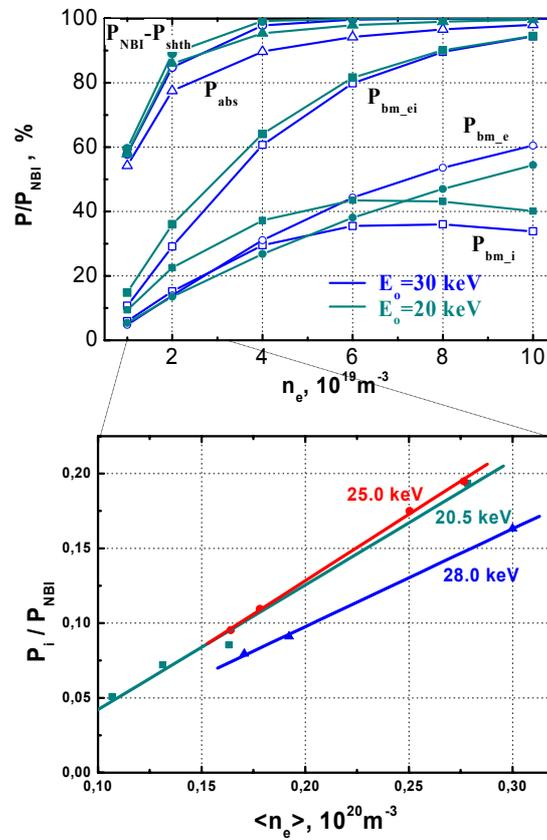
FIGURE 3. Deuterium beam power absorption. ASTRA code simulation (top), experimental data (bottom).
