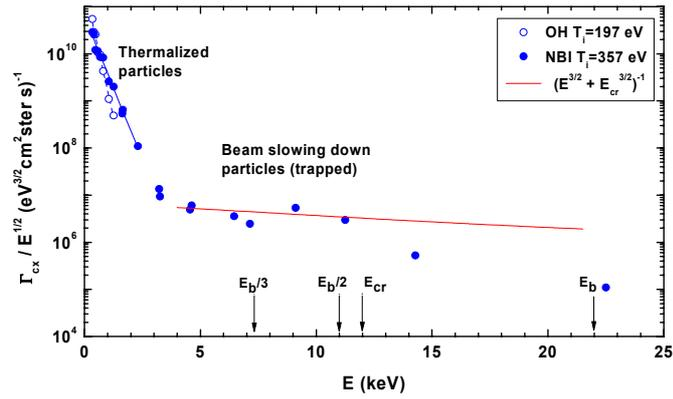
FIGURE 4. Energy spectra of charge-exchange neutrals emitted from plasma during NBI.  $E_{NB} = 22$  keV.
