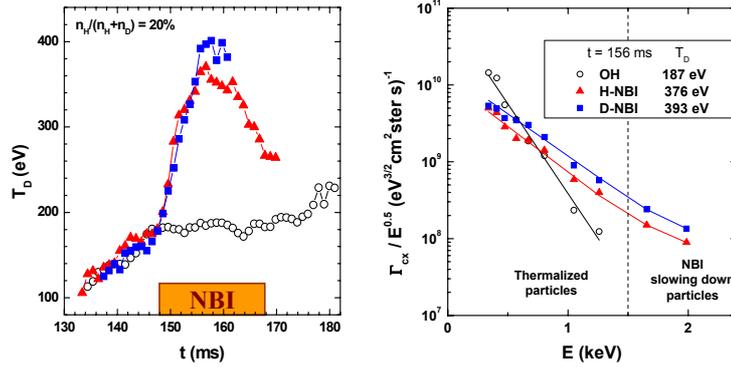
FIGURE 2. Comparison of hydrogen and deuterium beam injection. Ion temperature time evolution (left), charge-exchange deuterium energy spectra (right).  $P_{NB} = 0.6 \text{ MW}$ ,  $E_{NB} = 30 \text{ keV}$ ,  $I_p = 0.15-0.16 \text{ MA}$ .
