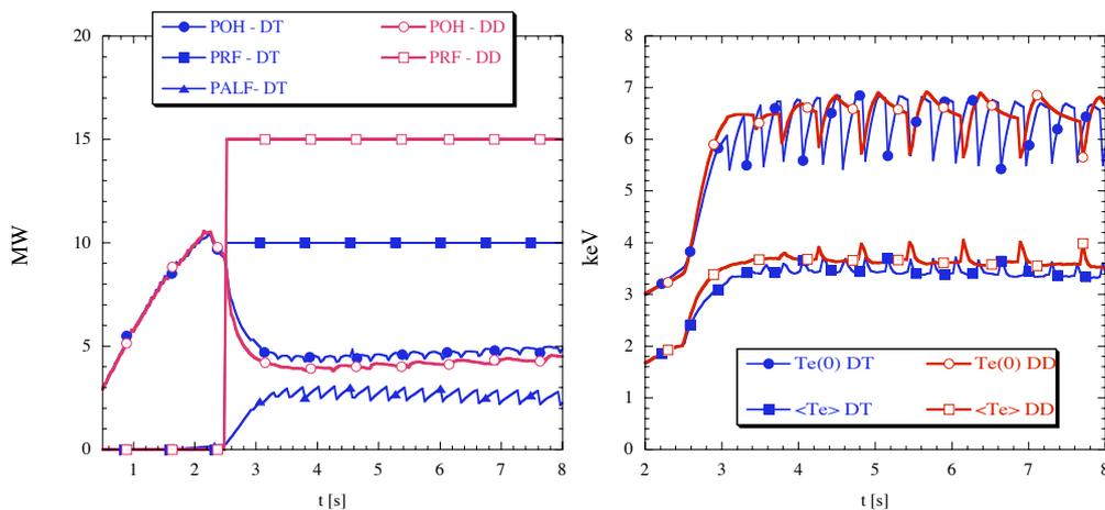
Fig. 1-Time evolution of powers (left panel) and temperatures (right panel) for a D-D and a D-T shot
