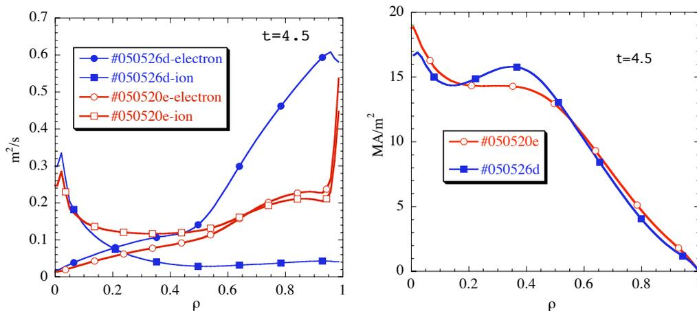
Fig.2 –Electron and ion thermal diffusivity profiles at 4.5s in the two shots (left panel). Current density profiles at the same time (right panel).
