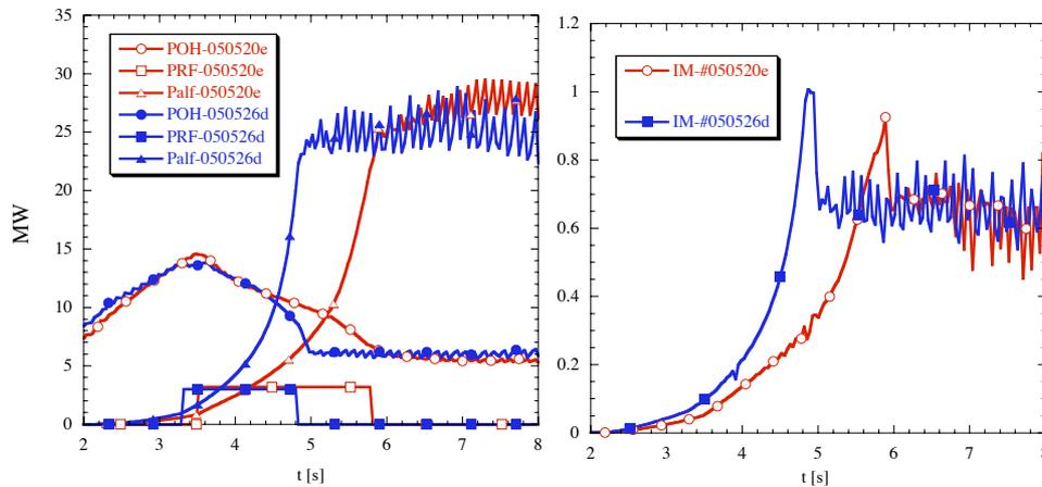
Fig.3-Time evolution of ohmic, RF and alpha power in the two shots (left panel). The ignition margin is in the right panel
