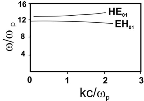
Fig3. Dispersion curves for waveguide modes
