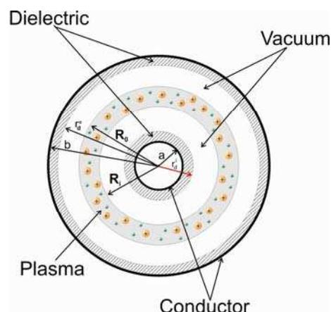
Fig1. Cross section of dielectric loaded plasma waveguide
