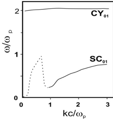
Fig2. Dispersion curves for space-charge and cyclotron modes
