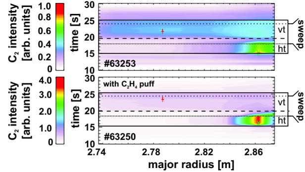
Figure 5: Radial distribution of the C<sub>2</sub> photon flux in the outer divertor measured with KT3.
