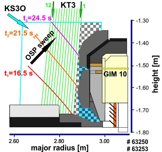
Figure 1: *Outer divertor: strike-point sweep and spectroscopic systems.*
