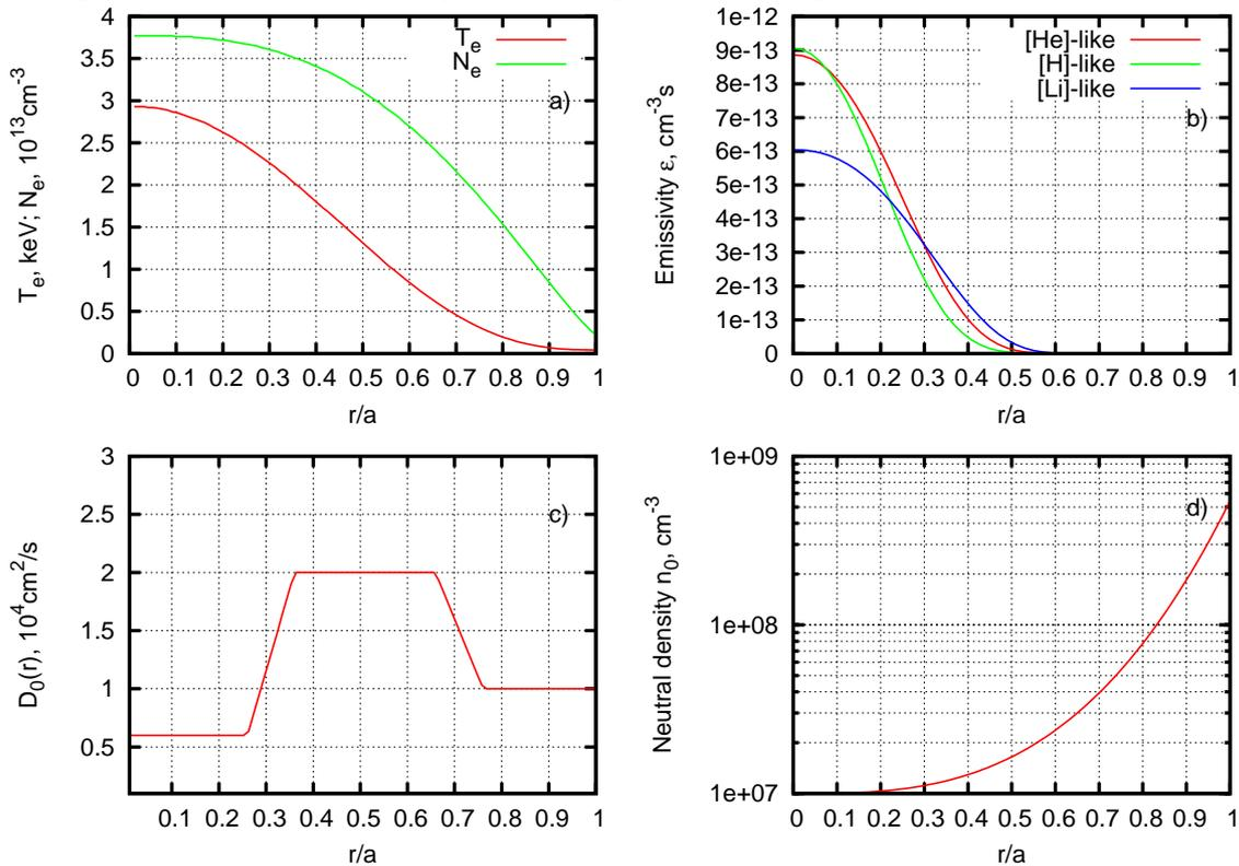
Fig.2 Radial profiles used in the model. <sup>a</sup> -electron temperature and density; <sup>b</sup> -emissivity of the ionization stages; <sup>c</sup> - diffusion coefficient; <sup>d</sup> - neutral density.
