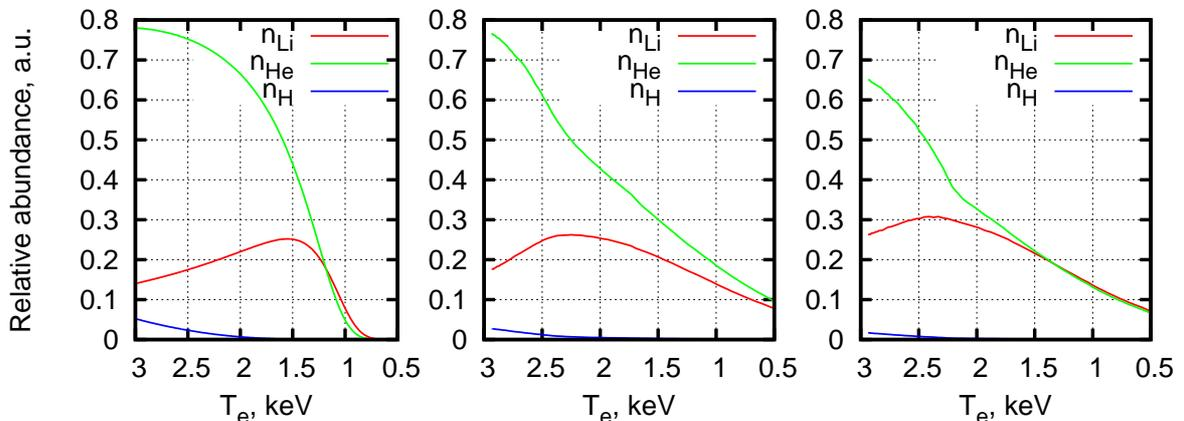
Fig.3 Ionization balance. <sup>a</sup>  $-k_D = k_n = 0$  (coronal equilibrium); <sup>b</sup>  $-k_n = 0, k_D = 1$ ; <sup>c</sup>  $-k_n = 5, k_D = 1$ .
