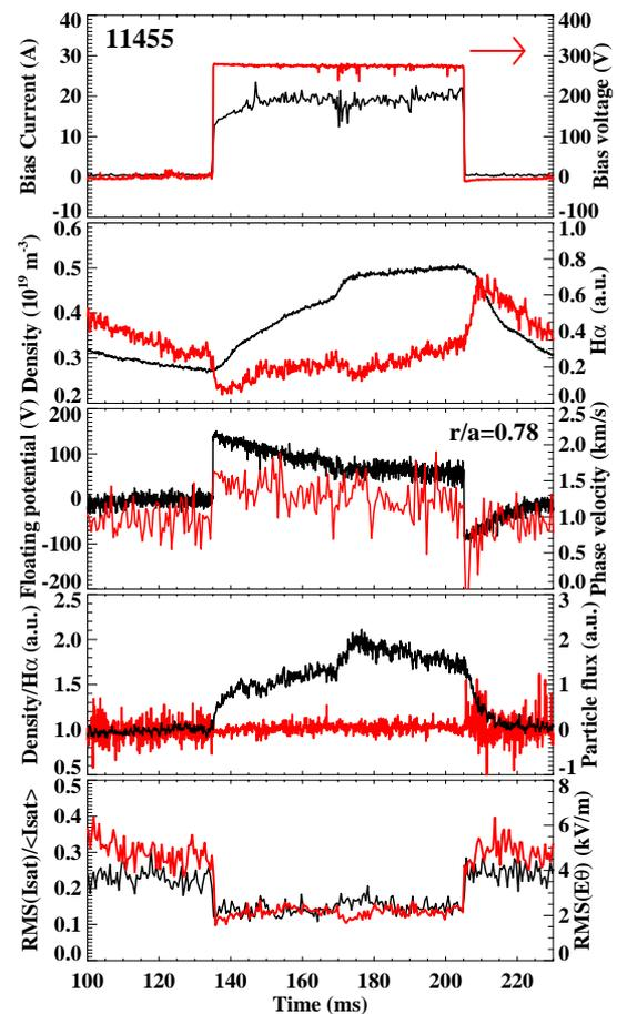
Figure 1: Time evolution of the main plasma parameters for a discharge with positive electrode bias at low density.
