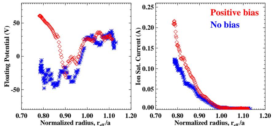
Figure 2: Edge radial profiles with and without electrode bias for a low density discharge.
