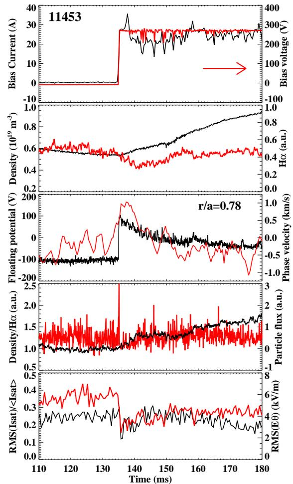
Figure 3: Time evolution of the main plasma parameters for a discharge with positive electrode bias at medium density.
