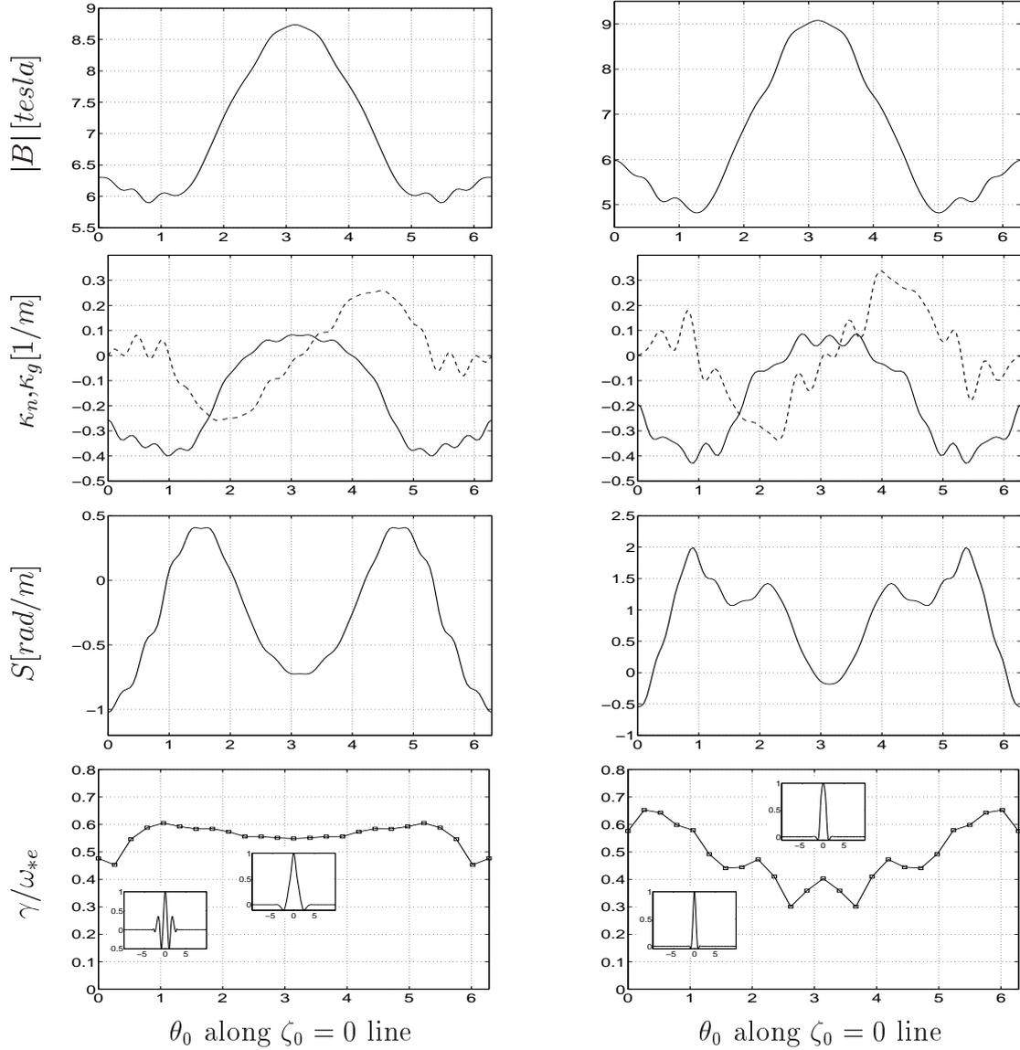
Fig. 1: Variation in the magnetic field strength  $|B|$ , the normal curvature  $\kappa_n$  (dotted curve), the geodesic curvature  $\kappa_g$  (solid curve), the local magnetic shear  $S$ , and the normalized growth rate  $\gamma/\omega_{*e}$  as a function of  $\theta_0$  for  $s = 0.4$  (left) and  $s = 0.7$  (right). The other parameters are:  $b = 0.1$ ,  $\tau = 1$ ,  $\epsilon_n = 0.1$ ,  $\eta_i = 3.0$  and  $\theta_k = 0$ .
