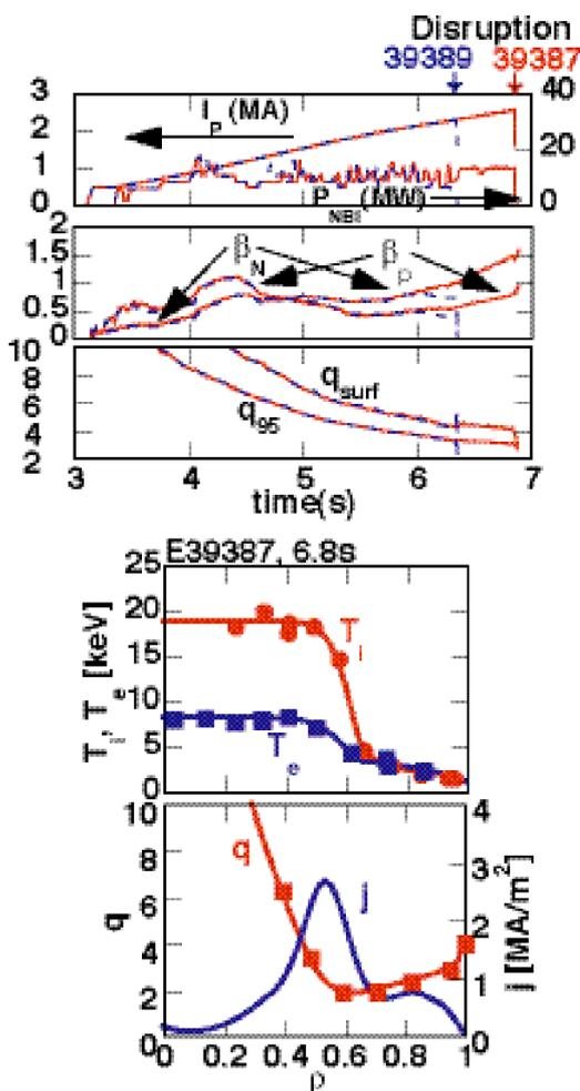
Fig. 1 Time evolution of (a)  $I_p$  and NB power, (b) normalized beta and poloidal beta, (c)  $q_{surf}$  and  $q_{95}$ . Radial profiles of  $T_i$  and  $T_e$  (c) and  $q$  and  $j$  (d) just before disruption of E39387 at  $t \sim 6.8s$ .
