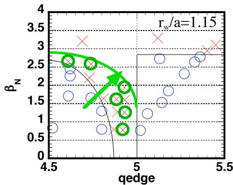
Fig. 10 The stability diagram for an extremely RS plasma with conducting wall at  $r_w/a=1.15$  (green curve and circles).
