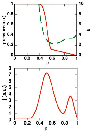
Fig. 6 The input profile for the ideal stability calculation . (a)Pressure and q, (b) toroidal current.
