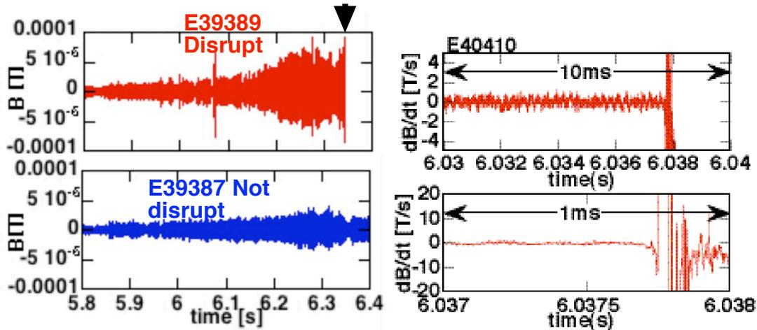
Fig. 4 (a) Temporal evolution of magnetic fluctuations in disruptive shot (upper) and no disruptive shot (lower). The  $m/n=4/1$  mode starts at  $t \sim 6.1s$ . (b) Magnetic fluctuation before disruption of E40410. No precursor was detected.
