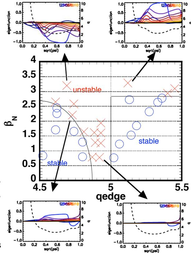
Fig. 7 The stability diagram for an extremely RS plasma with the profiles shown in Fig. 6.
