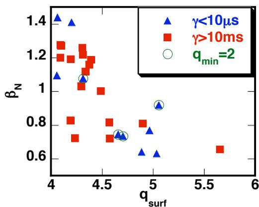
Fig. 5  $\beta_N$  vs  $q_{eff}$  at disruptions with the continuous change of pressure gradient of precursor (blue triangle) and without the rational surface, which is determined by the precursor (red square). The green open circles denote  $q_{min}=2$ .
