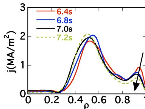
Fig. 2 Temporal evolution of plasma current. The peripheral plasma current decreases after stopping current ramping up
