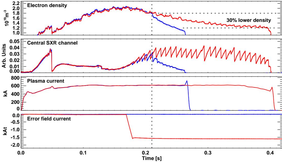
Figure 4: Time traces for shots with (red) and without (blue) error field correction.
