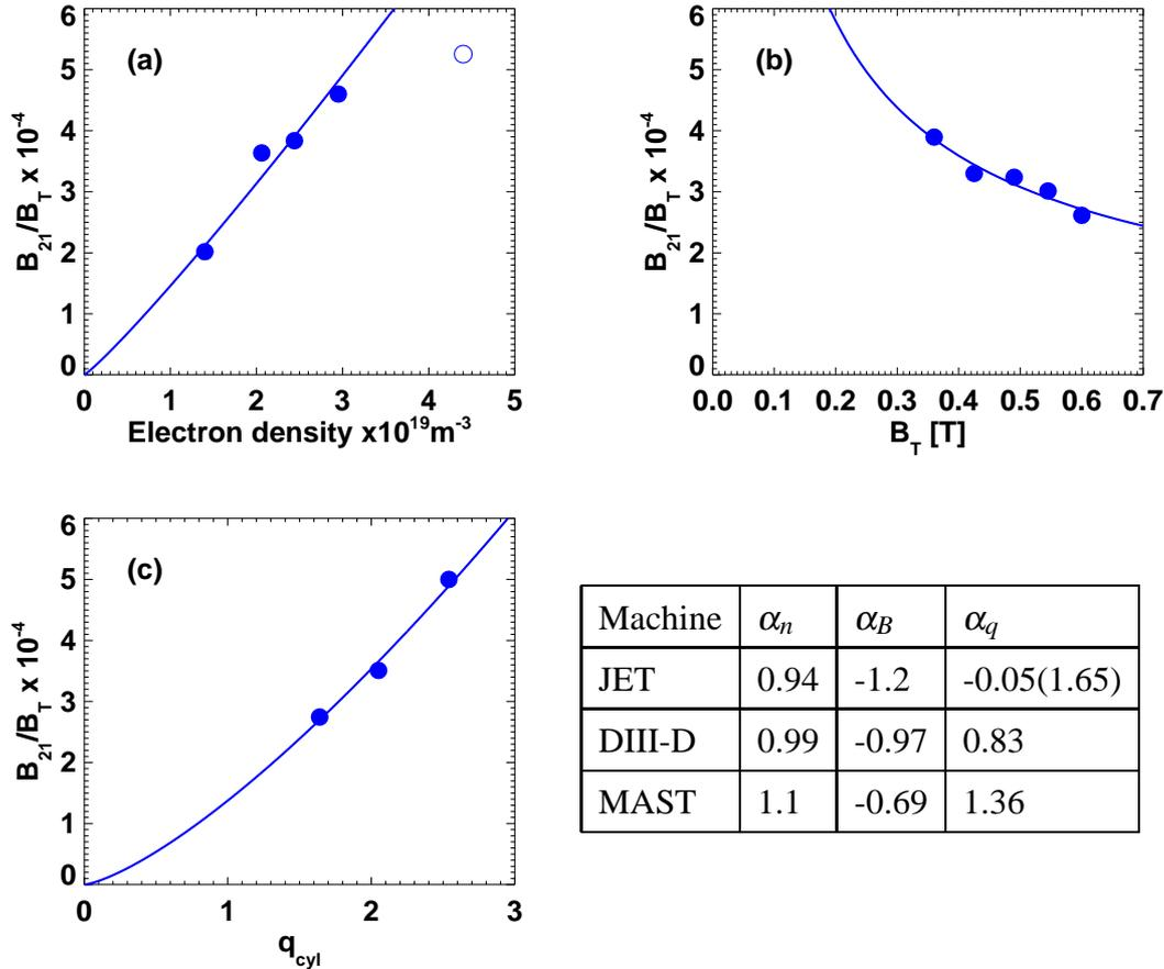
Figure 5: Scaling of the locked mode threshold with density, toroidal field and  $q_{cyl}$ .
