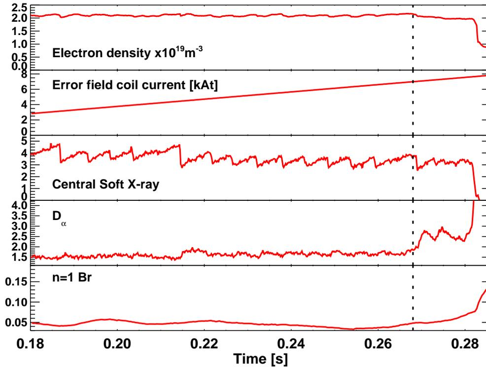
Figure 2: Time traces for a typical shot. The onset of the locked mode is indicated by a sudden drop in the electron density, the disappearance of the sawteeth and a rise in the  $D_\alpha$  emission at the divertor.
