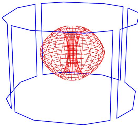
Figure 1: The MAST error field coils
