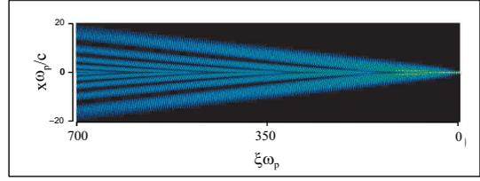
Figure 2: Distribution of the magnetic field  $B_y$  behind the laser pulse.
