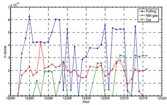
**Figure 2.** Injected particles by the puffing valve (blue stars) and NBI (green triangles) and released ones, measured by the quadrupole analyzer (red circles).
