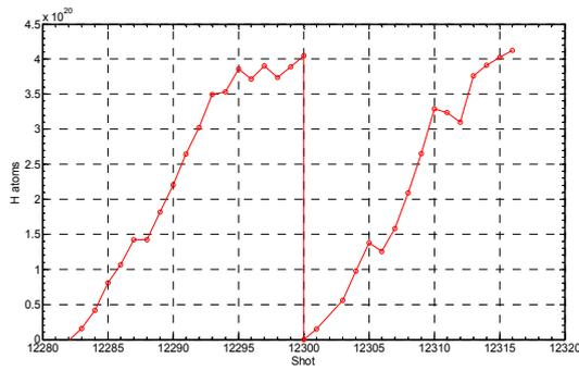
**Figure 1.** Total particle inventory. At shot 12300 He Glow Discharge. Density cut-off in last pulses before and after glow.
