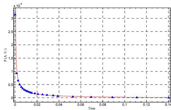
**Figure 6.** Outgassing after a shot. Experimental points and fitting ( $t^{-0.7}$ )
