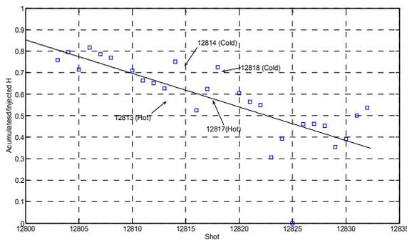
**Figure 3.** Evolution of ratio between accumulated particles and incoming flux. The figure also shows how cold dense plasmas accumulate more hydrogen than that hot ones.
