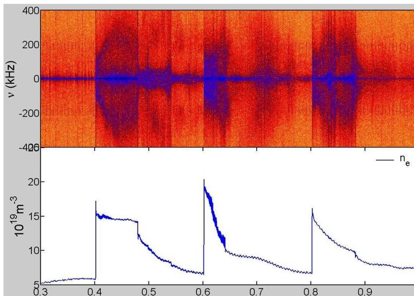
Figure 1: FTU pulse 27943. Reflectometry spectrogram during multiple pellet injection. The turbulence properties differ during good and bad particle confinement
