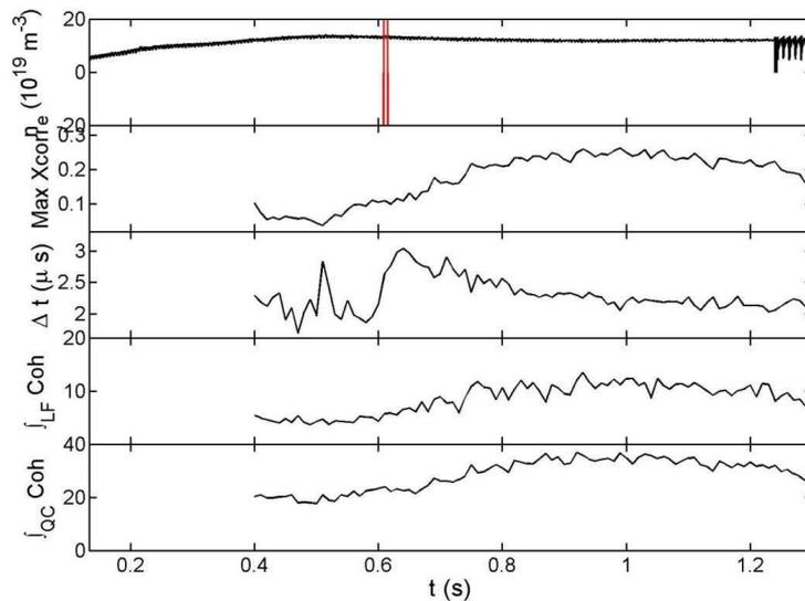
Figure 4: FTU shot 25500. Evolution of turbulence properties during RI mode phase. a) electron density. b) Max of cross correlation function. c) Delay between 2 channels. d,e) Coherency of LF and QC components
