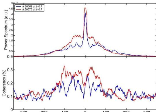
Figure 2: Comparison of spectra and coherency for two discharges (26669-Blue, with ITB and 26672-Red without ITB)
