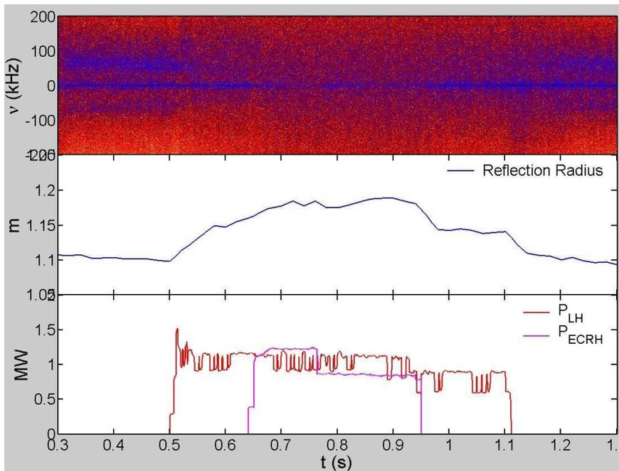
Figure 3: FTU shot 27749. a) Reflectometry signal spectrogram. b) Reflection radius. c) Additional heating
