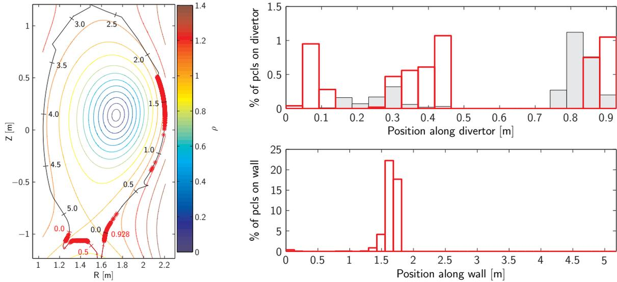
Figure 3: Fast particle (60 keV) losses to the divertor and wall structures. The poloidal cross section on the left illustrates the wall and divertor coordinates used in the histogram on the right and in figures 4 and 5. The red asterisks show the hit points in the presence of ripple. In the histogram, red and grey bars show the results with and without ripple, respectively. The percentages don't add up to 100% because the thermalized particles don't show up in the histogram.
