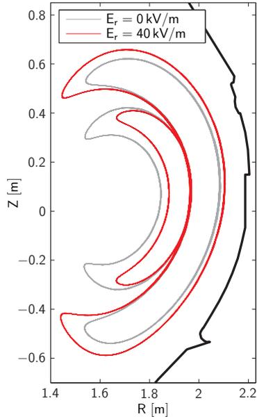
Figure 1: Effect of a constant radial electric field on orbit widths.
