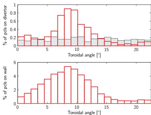
Figure 4: Toroidal variation of the fast particle losses. Red and grey bars are as in figure 3.
