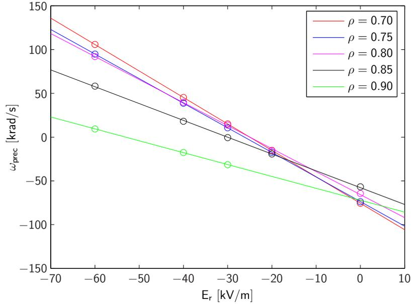
Figure 2: Effect of a constant radial electric field on the precession drift frequency (positive sign indicates co-injection direction) for different birth radii.
