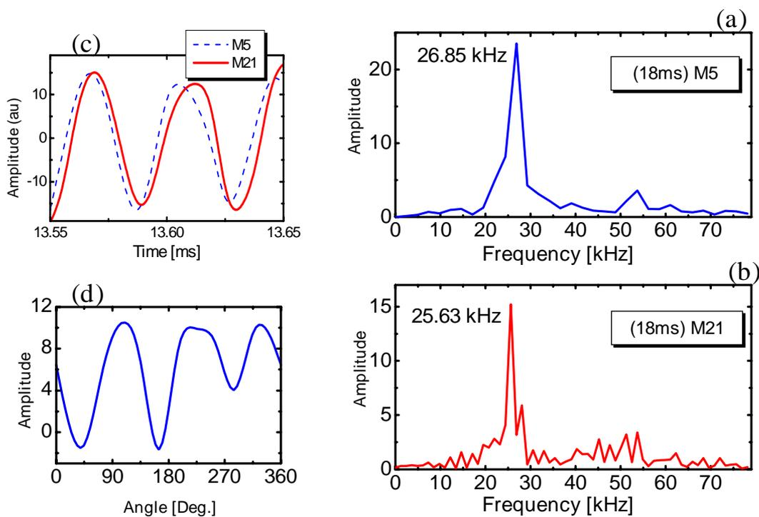
Fig.3-(a, b) The arbitrary time selection of magnetic oscillations frequency detected by M5 and M21 Mirnov coil positioned according to fig.1. (c) Signals of magnetic coils oscillations. (d) A spline fit of the amplitude data taken from each coil at the same time, the poloidal angular dependence of Mirnov coil signals from shut no.1112.13
