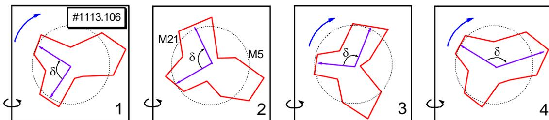
Fig.2- The detailed time evolution of poloidal variations of  $m=3$  mode diagram. The M21 and M5 indicate the Mirnov coils position according to fig.1. The angle of  $\delta$  indicates the lobe angle of mode diagram which changes during rotation.
