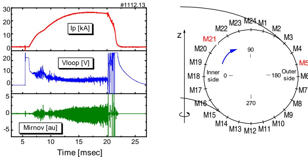
Fig.1- a) The Mirnov coils array and their positions, b) The time evolution of plasma current, loop voltage and Mirnov coil oscillations.
