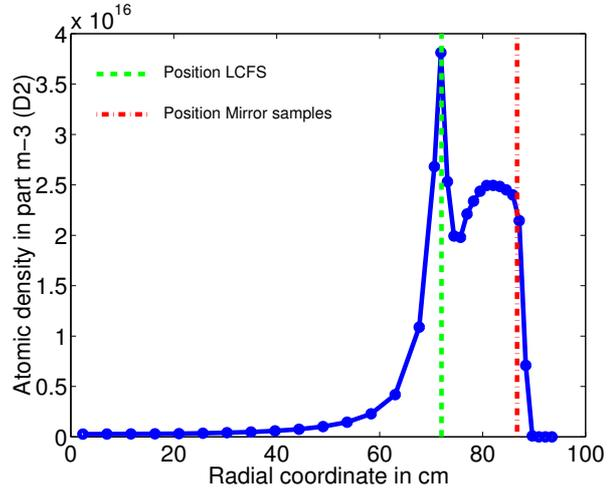
**Figure 2:** Eirene code: Radial particle distribution. Contributions from two sources at different radial positions (recycling at the CIEL limiter roof and recycling at the main chamber) are superimposed.
