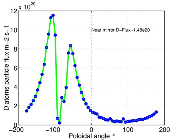
**Figure 1:** Eirene code: Deuterium flux – the mirrors are positioned at a poloidal angle of  $-180^\circ$ .
