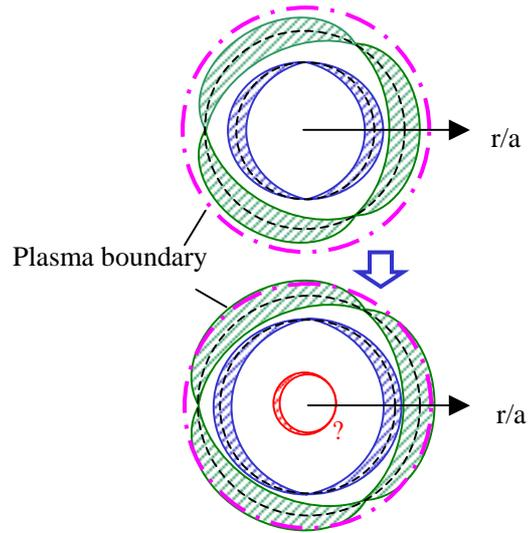
Fig. 7: The change of poloidal magnetic surface until current quench.
