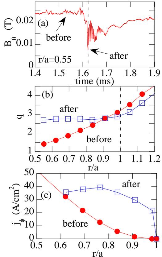
Fig. 6: (a) Internal magnetic field at the core region. (b), (c) The safety factor profile and current density profile before and after current quench.
