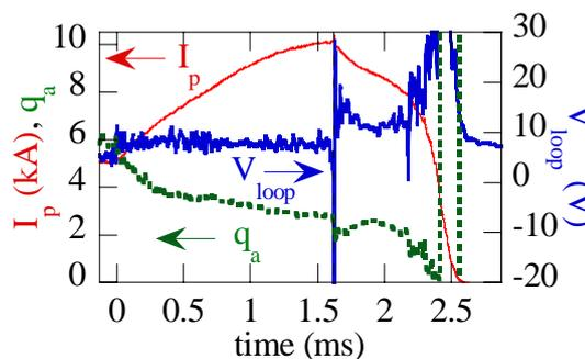
Fig. 1: Typical disruption waveform in HYBTOK-II ( $Bt \sim 0.25$  T).
