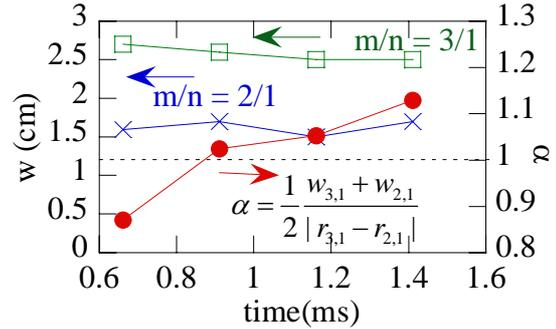
Fig. 5: Temporal evolution of magnetic island width and the stochasticity parameter  $\alpha$  during current ramp-up phase.
