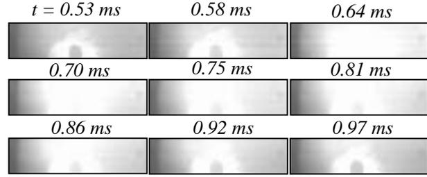
Fig. 4: The measurement of total light emission by using high-speed camera with 18000 fps
