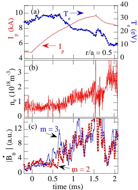
Fig. 3: (a), (b) Temporal evolution of electron temperature and density during thermal quench. (c) Poloidal mode analysis.
