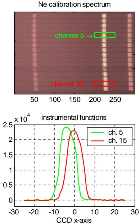
Figure 2. Typical full frame Neon calibration spectrum. Selected zones are used to define instrumental functions for the 2 channels.
