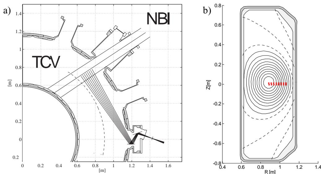
Figure 1. (a) CXRS experimental setup in horizontal cross-section of TCV. (b) Flux surfaces for a typical L-mode shot in limited configuration. CXRS measurement points are highlighted in red.
