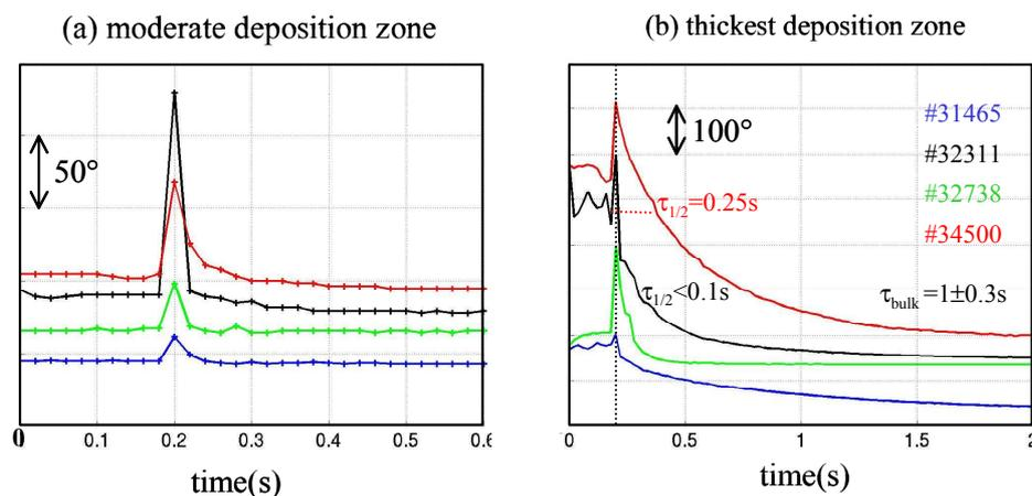
**Figure 2:** Temperature as measured by the IR wide angle camera on the moderate (a) and the thickest (b) deposition zone. Data have been artificially synchronized and shifted in the temperature scale to make the comparison easier.
