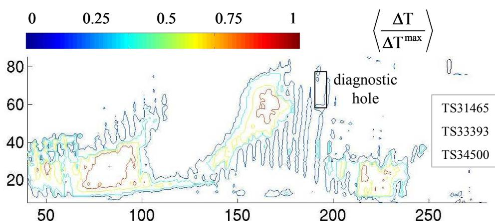
**Figure 3:** Average of the normalized  $\Delta T$  measured during a small, a medium and a strong disruption.
