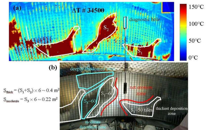
**Figure 1:** (a) Increase of temperature on the TPL during the disruption as measured by the wide angle IR camera. (b) Same part of the TPL without plasma.
