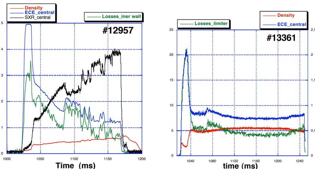
**Fig. 3.** Fast transitions at the plasma core as observed at (left) plasma wall and (right) the limiter.
