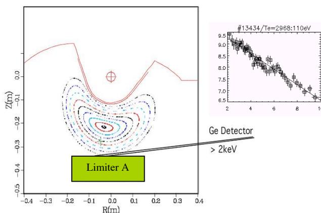
**Fig. 2.** Schematic view of the Ge detector location and a typical spectrum in the range of 2 keV to 10 keV
