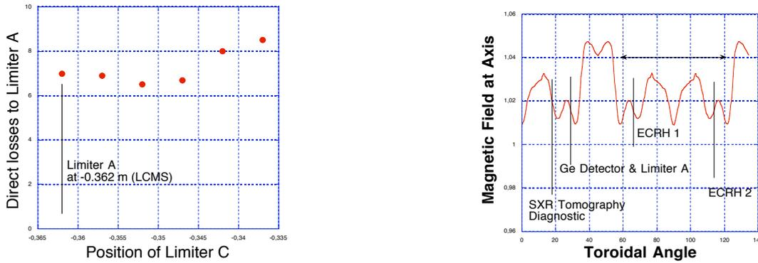
**Fig. 4.** (left), Intensity of direct losses at limiter A while introducing the limiter C inside the plasma. (right), Magnetic field at axis. Also shown the diagnostic and the microwave injection ports positions.
