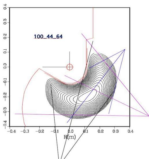
**Fig. 1.** Schematic view of the tree inner SXR cameras.
