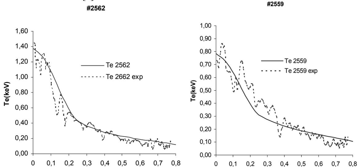
**Figure 2.** Electron temperature profile simulations of shots #2562 and #2559 made with the model previously described
