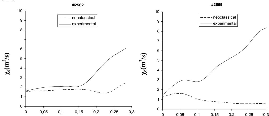
**Figure 4.** Comparison of anomalous and experimental electron diffusivities profiles at the plasma centre in #2562 shot (left) and #2559 shot (right)
