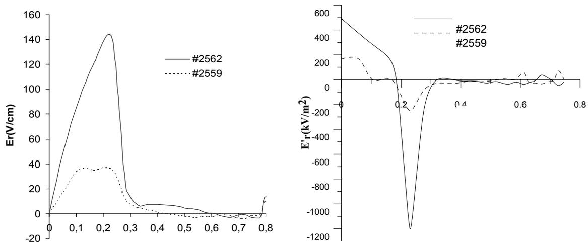
**Figure 3.** Calculated electric field profile in the case of #2559 and #2562 shots (left). Derivative  $E_r$  profile which gives  $E \times B$  shear flow (right)
