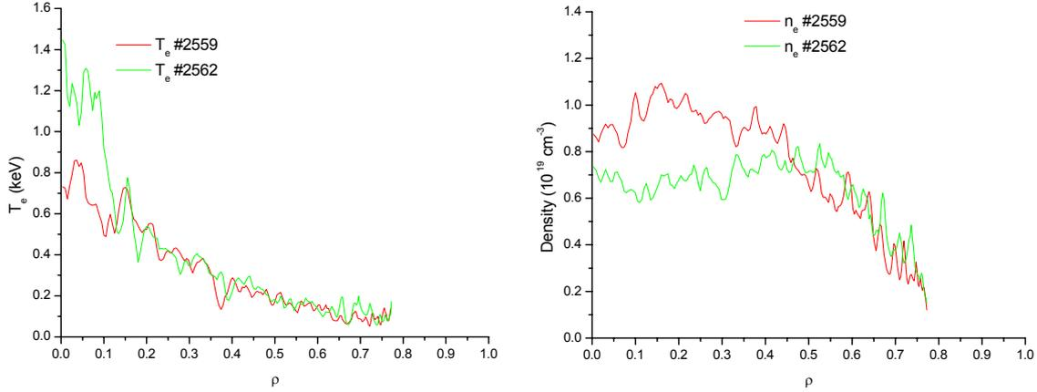
**Figure 1.** Electron temperature and density profiles collected from Thompson scattering in #2559 and #2562 shots.
