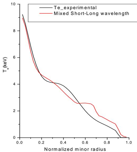
Figure 3 Comparison between mixed short wavelength long wavelength model and experimental electron temperature profile.
