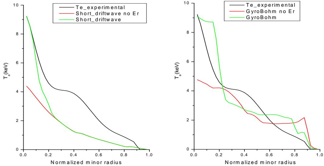
Figure 2 Comparison between short wavelength model (left), GyroBohm model (right) and experimental electron temperature profile, with and without electric field shear effect.
