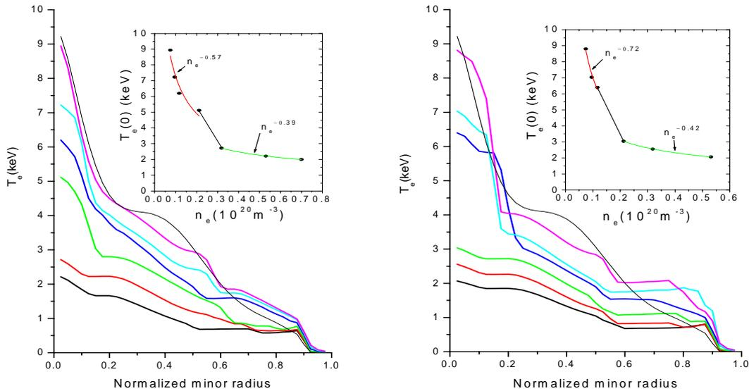
Figure 4 Electron temperature profiles obtained with mixed model (left) and with GyroBohm model (right) for the different average densities appearing in the upper figure.
