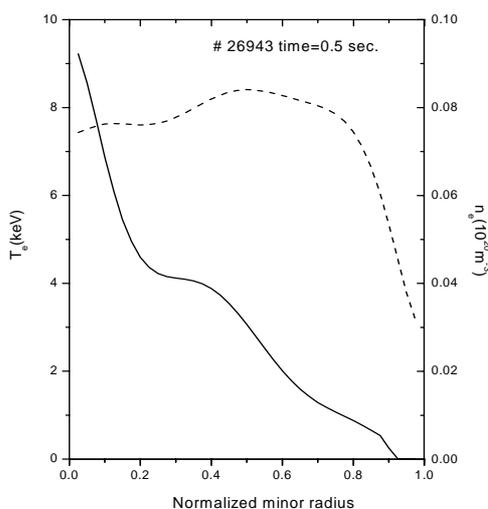
Figure 1 Experimental profiles of electron temperature (solid) and density (dashed) obtained in LHD
