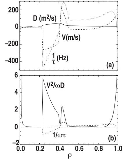
Fig. 3. (a) Evaluation of  $D$ ,  $V$ ,  $1/\tau$ , for the critical gradient model [Eq. (13)] vs normalized radius. The co-efficients used are the same as for AUG [2]. The kinetic profiles are those measured in the same plasma shown in Fig. 2. The reciprocal of the dimensionless parameters from the x-axes on Fig. 1 are shown in (b).
