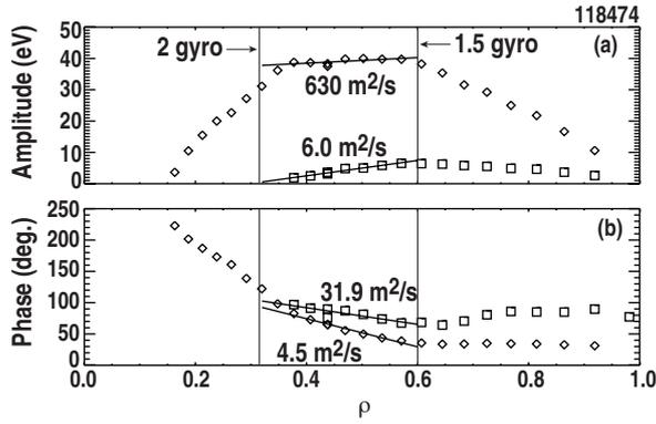
Fig. 2. (a) Amplitude and (b) phase of the heat pulse vs. normalized radius for the fundamental (diamonds) and third harmonic (squares) frequency in the case with two gyrotrons heating at  $\rho=0.32$  and one continuous and one modulated gyrotron heating at  $\rho=0.6$ . The lines show the linear fits used to determine  $D_{\text{amp}}$  and  $D_{\text{ph}}$ .
