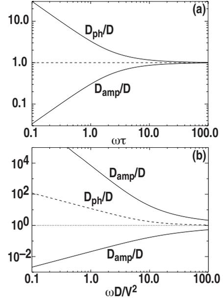
Fig. 1. Slab estimates of diffusivity for the case of (a) diffusion plus damping and (b) diffusion plus convection. The upper curve in (b) is for the case of the heat pulse moving in the direction of the convection.
