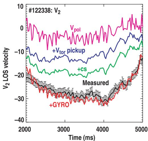
Fig. 5. Measured LOS velocity (black) of V2 chord ( $\rho \sim 0.25$ ), showing the contribution as additional physics comprising this measurement is included: Poloidal rotation (magenta), toroidal rotation pickup (blue), cross-section correction (green), and gyro-correction (red).
