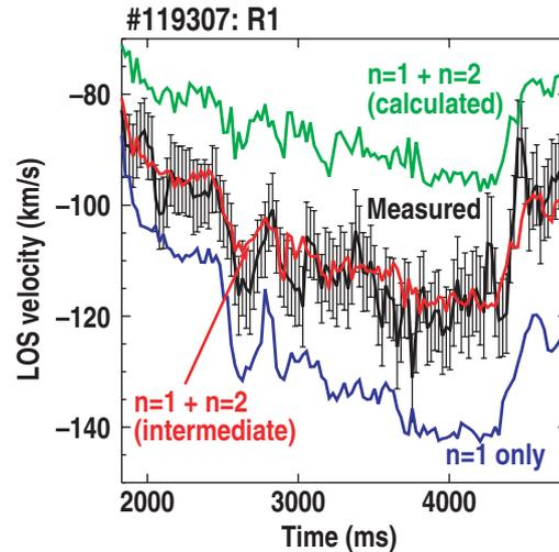
Fig. 2. Measured LOS velocity for a radial chord (black), with reconstructed value based on  $n=1$  cross-section only (green), effective cross-section using calculated  $n=2$  fractions (blue), and intermediate cross-section (red).
