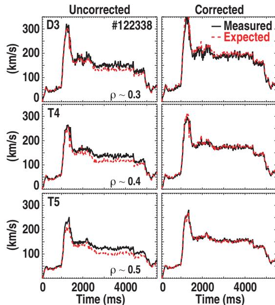
Fig. 3. Measured (black) LOS velocities of three tangential chords [ $\rho \sim (0.3, 0.4, 0.5)$ ] and the expected values (red) based on interpolation from chords with different viewing geometry. On the left, the uncorrected LOS velocities show that the measurement sets do not lie on the same smooth curve, but after correction on the right, the agreement is good.
