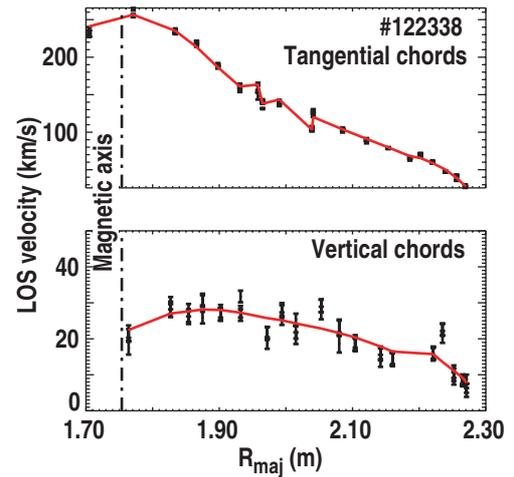
Fig. 4. Measured LOS velocities for (a) tangential and (b) vertical viewing CER chords. The red points are the measured values with error bars, while the black squares are the re-projected LOS velocities after solving for the toroidal and poloidal rotation. The jaggedness in the tangential profile arises because the chords view the plasma from two distinct ports with different toroidal angles.
