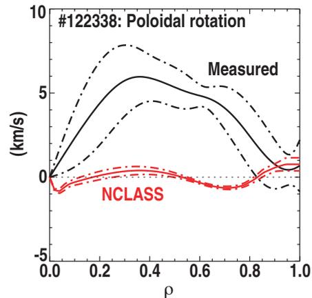
Fig. 6. Corrected poloidal rotation profile [black], averaged over an ELM-free period between 3000–4000 ms, compared with the neoclassical prediction from NCLASS averaged over the same period. The dashed bands represent the error estimate, obtained from the standard deviation of the time resolved profiles during the time window.
