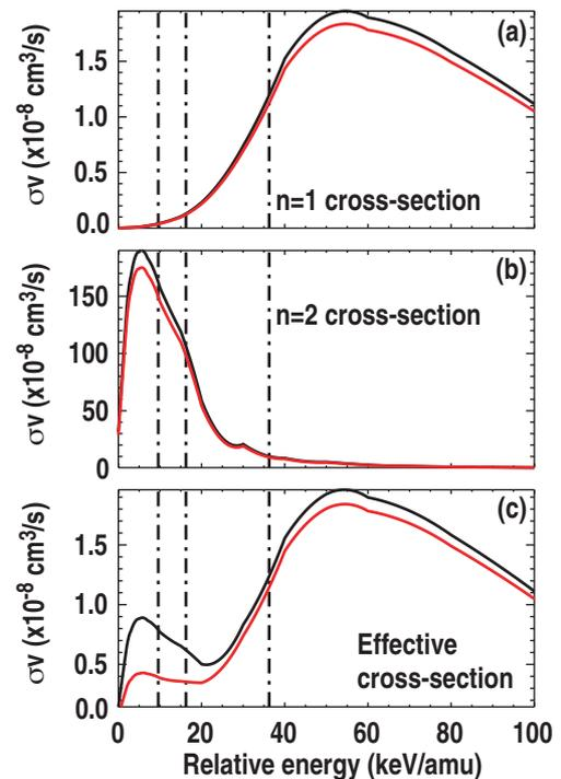
Fig. 1. Distortion of effective charge exchange cross-section in the presence of excited beam neutrals at 2 radial locations: on-axis (black) and mid-radius (red) for a typical set of plasma parameters. (a)  $n=1$  capture cross-section, (b)  $n=2$  cross-section, (c) effective cross-section taking into account relative  $n=2$  contributions.
