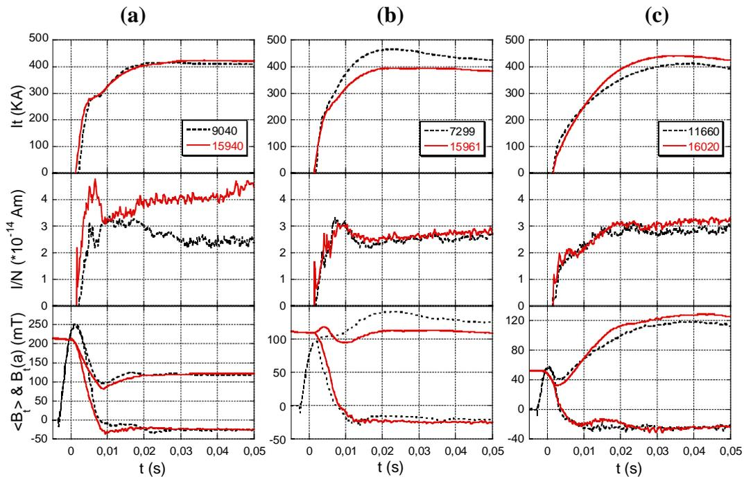
*Fig.1 Plasma current, I/N ratio, toroidal field (mean and edge) for pulses with different RFP setting-up in RFX (black line) and RFX-mod (red line): (a) aided, (b) matched and (c) ramped. In all cases both the time evolutions and the final states are very similar.*
