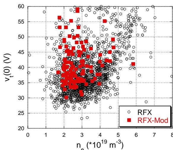
Fig.3 Resistive loop voltage versus density for pulses at 600 kA
