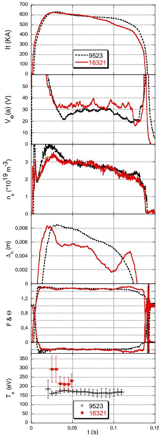
Fig.2 Reference "long pulses" in RFX (9523) and RFX-mod (16321). Both discharges terminate because of the turning off of the voltage at 0,11 and 0,12 s respectively.
