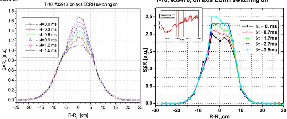
Fig.1. Time evolution of SXR radial distribution, after switching on central ECRH.
