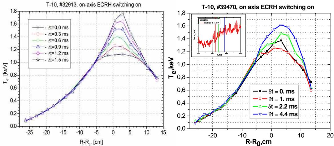
Fig.2  $T_e$  evolution after switch-on of central ECRH in the OH phase in two shots.
