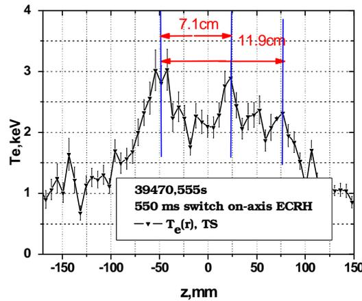
Fig.3  $T_e$  (TS) in OH and 4 ms after on-axis ECRH. fig.4  $T_e$  (TS) at 5ms after switch-on of on-axis ECRH.
