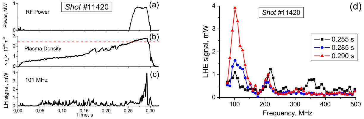
Fig. 1: a) RF power injected into the plasma, b) line integrated density, c) lower hybrid emission (LHE) signal measured at 101 MHz, d) LHE spectrum measured at different time slices.
