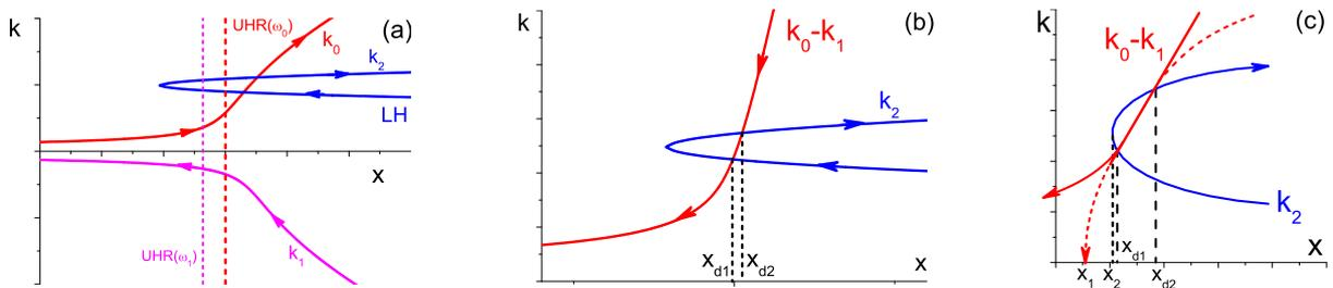
Fig. 2: a), b) dispersion curves for pump UH wave  $k_0$ , reflected UH wave  $k_1$  and LH wave  $k_2$ . Arrows denote group velocity direction. c) Three-wave interaction, when two waves possess turning points.
