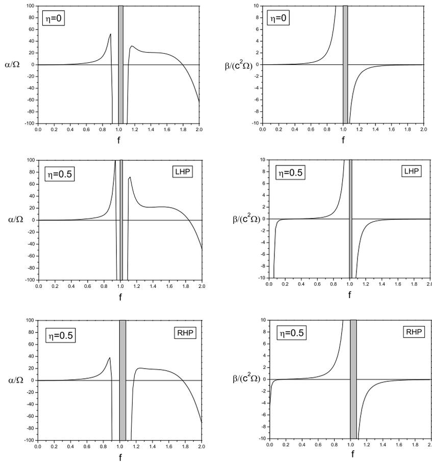
Figure 2: The nonlinear ( $\alpha$ ) and dispersive ( $\beta$ ) coefficients of the NLS equation, as a function of frequency, for  $\eta = 0$ , and for  $\eta = 0.5$  and left-hand polarized waves, and for  $\eta = 0.5$  and right-hand polarized waves.
