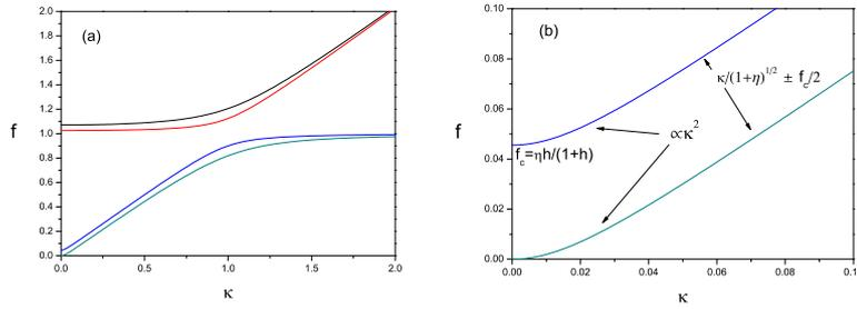
Figure 1: Linear dispersion relation for electromagnetic waves in a pair plasma. (a) Full frequency range, (b) small frequency.
