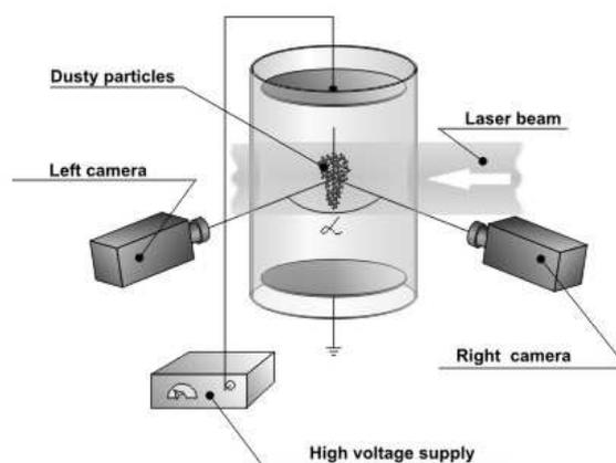
Fig. 1. Experimental setup scheme.
