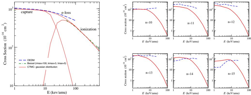
Figure 2: (a) Total capture and ionization cross sections for the  $Ne^{10+} + H(2s)$  collisions. b) Partial semiclassical(- -) and classical-CTMC(—) capture cross sections to  $n=10 - 15$  states.
