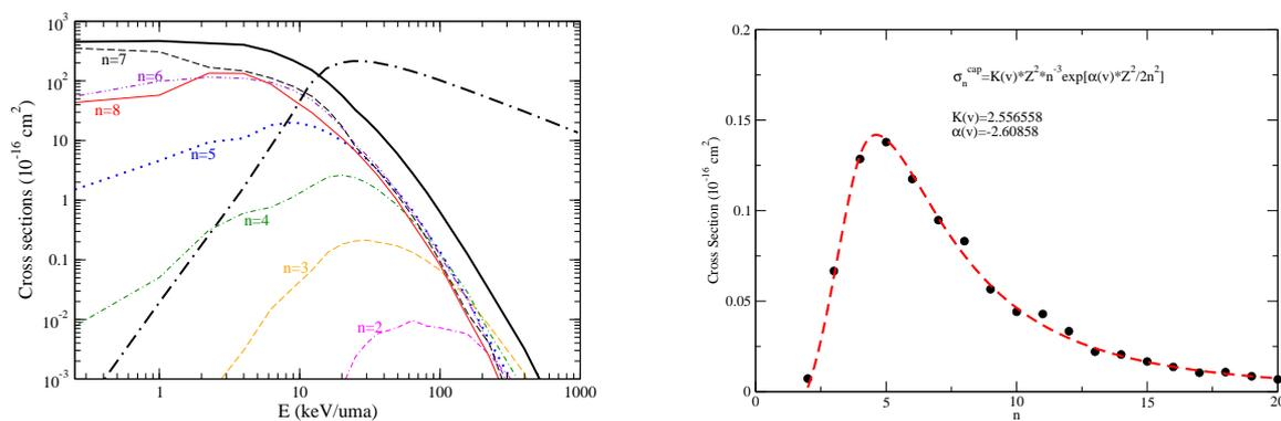
Figure 3: a)  $B^{5+}+H(2s)$  total capture (—) and ionization (— · —) together with the  $n$ -partial ( $n = 2 - 8$ ) capture recommended cross sections as a function of the impact energy. b) Oppenheimer  $n^{-3}$  extrapolation law for  $E \sim 100keV/amu$ .
