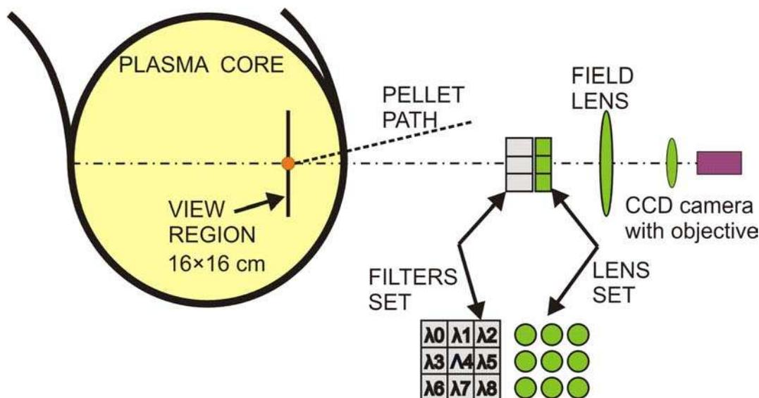
Fig. 1. Layout of NIOS measurements in LHD.
