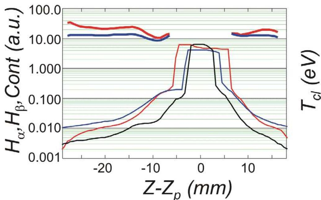
Fig.4. Toroidal intensity profiles  $I_{H\alpha}(0,z)$  (thin red),  $I_{H\beta}(0,z)$  (thin blue),  $I_{Cont}(0,z)$  (thin black) in the #65303 LHD shot. Evaluated  $T_{cl,H\alpha}(0,z)$  (thick red) and  $T_{cl,H\beta}(0,z)$  (thick blue) profiles are shown as well.
