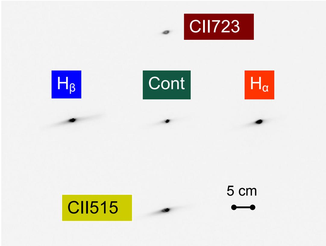
Fig. 3. Sample of NIOS measurements in the #65303 LHD shot. Exposure time is 10  $\mu$ s. NIOS is triggered at  $R = 4.3$  m.
