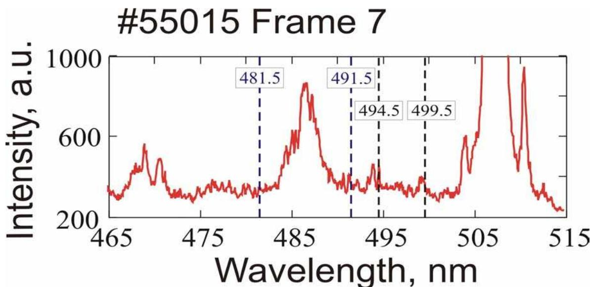
Fig. 2. Sample of time-resolved wide-view angle spectral measurements of TESPEL ablation cloud [7] for choosing the H $\beta$  and Continuum filter parameters.
