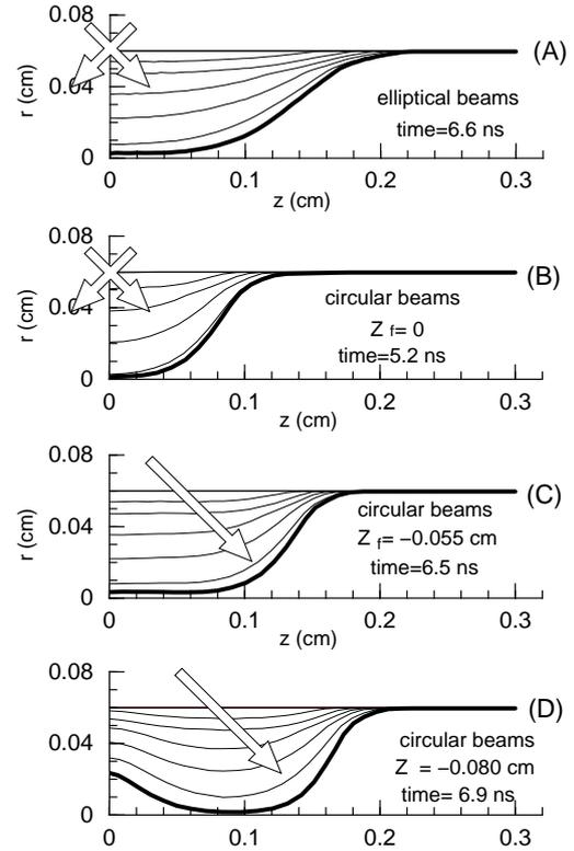
Figure 4: Evolution of the gas-ablator interface.
