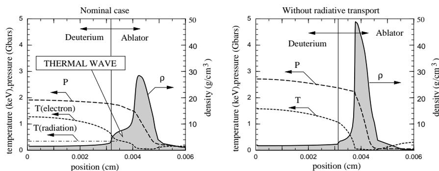
Figure 5: Final compressed configuration with and without radiative transport enabled
