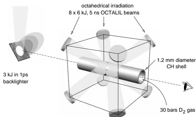
Figure 1: OCTALIL cylindrical target
