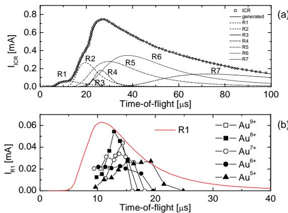
Fig. 2 Deconvolution of a current of  $\text{Au}^{q+}$  ions produced by a Nd:YAG ( $\lambda=1064$  nm,  $I_L = 3 \times 10^{10}$  W/cm<sup>2</sup>) – (a). Comparison of the  $\text{Au}^{5+}$  to  $\text{Au}^{9+}$  ion currents reconstructed from the cylindrical electrostatic analyser spectra with the recovered peak R1 – (b).
