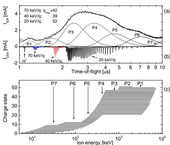
Fig. 3 Deconvolution of an ion collector signal to seven current peaks – (a). CEA spectra of  $\text{Au}^{q+}$  ions with  $E_{\text{ion}}/q = 20$  keV/q, 40 keV/q, and 70 keV/q having  $q_{\text{max}} = 52, 39,$  and  $42,$  respectively – (b).  $q - E_{\text{ion}}$  spectrum of  $\text{Au}^{q+}$  ions emitted from a plasma produced with intensity of  $5 \times 10^{14}$  W/cm<sup>2</sup>. The arrows show the positions of the recovered peaks – (c).
