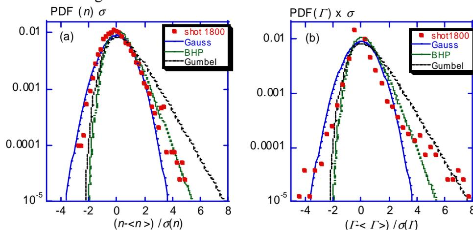
Figure 4. Rescaled density fluctuation pdf (a) and flux fluctuation pdf (b) for the shot 1800 ( $r = 0.1$  cm;  $P_{LMG} = 0.6$  kW,  $B = 0.12$  T). For comparison we show the standard Gauss distribution, the BHP distribution and a Gumbel distribution
