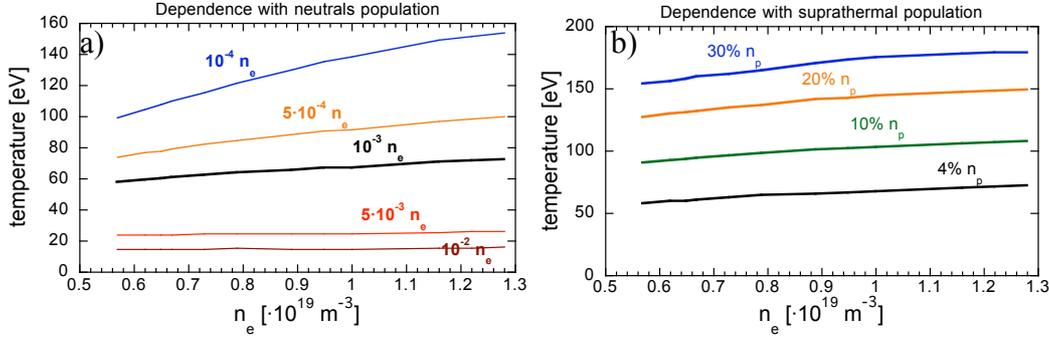
Fig. 3. Model results showing the influence on the temperature of: (a) neutral density and (b) the suprathermal population.
