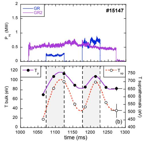
Fig. 4. (a) Power injected to the plasma with two gyrotrons: one fixed, the other alternating pulses. (b) Spectroscopy results obtained from  $H_\alpha$  line.
