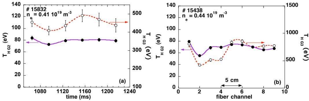
**Fig. 2.** (a) Temporal evolution of the temperature for G2 (solid circles) & G3 (open circles) measured in the parallel direction.(b) Spatial distribution of the temperature for G2 (solid circles) & G3 (open circles) measured in the perpendicular direction.
