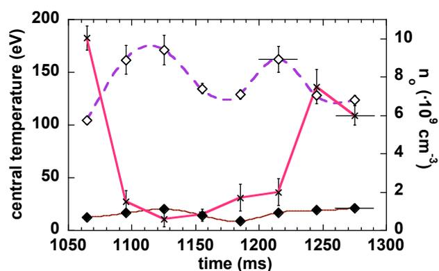
Fig. 5. Left axis: central temperatures deduced with (open diamonds) and without (solid diamonds) suprathermal population. Right axis: neutrals density (crosses) necessary to explain the experimental results.
