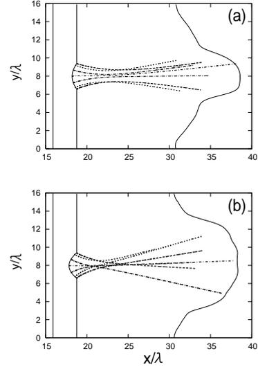
Fig. 4: Proton beam trajectories and contour of (a)  $D=0.6\lambda$  and (b)  $D=\lambda$  from a parabolic concave target at  $\omega t=800$ .
