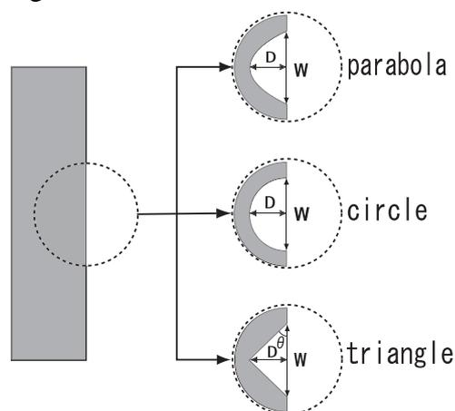
Fig. 1: The geometry of the target containing the concave cavity.
