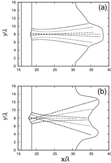
Fig. 2: Proton beam trajectories and contour of (a)  $D=0.4\lambda$  and (b)  $D=\lambda$  from a triangular concave target at  $\omega t=800$ .
