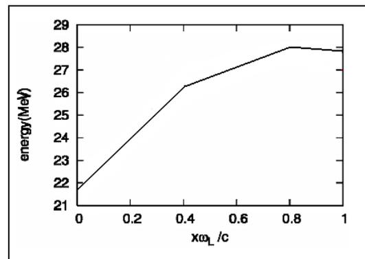
Fig.4. Maximum ion energy distribution from a elliptic concave target at  $D=0\sim 1.0 \mu\text{m}$ .
