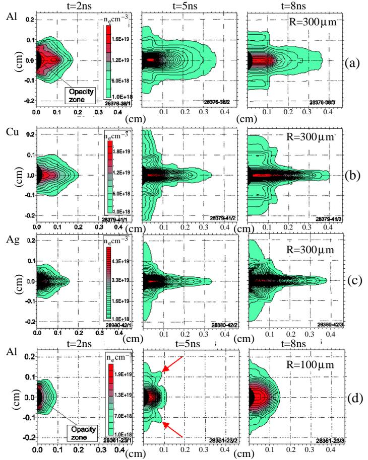
Figure 1: Experimental sequence of the electron density isolines at 2, 5, 8 ns for  $R_L = 300 \mu\text{m}$ ,  $E_L = 100 \text{ J}$  and the wavelength of  $0.438 \mu\text{m}$  for Al (a), Cu (b) and Ag (c) targets; (d) for  $R_L = 100 \mu\text{m}$  and Al target
