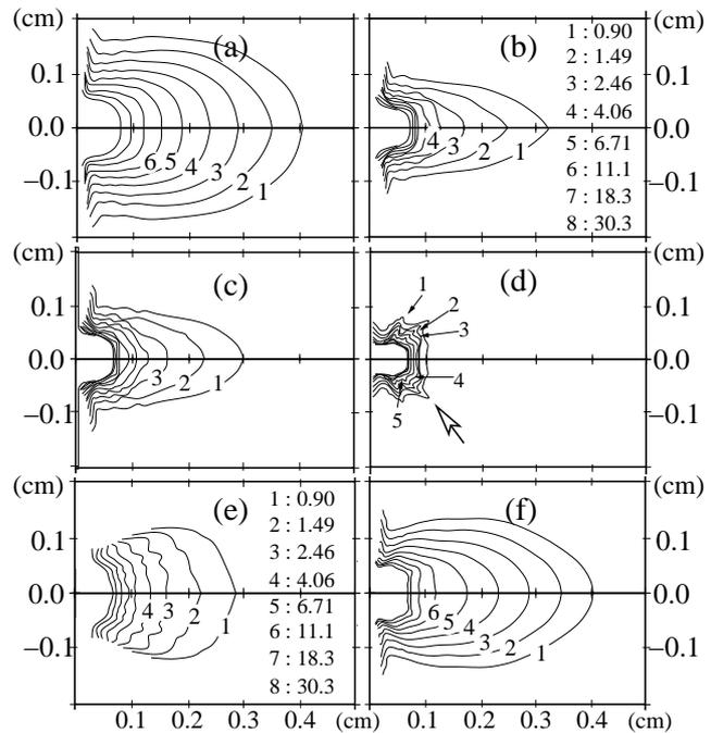
Figure 2: Electron density distributions at  $t = 5$  ns, for  $E_L = 100$  J,  $\tau_L \sim 400$  ps,  $\lambda_L \sim 0.438 \mu\text{m}$  and  $R_L = 300 \mu\text{m}$ . Without the radiation transport (a), with the radiation transport (b), with the magnetic fields (c), with a smaller laser spot radius (d), with a different energy distribution the the focal spot (e) and with an aluminium target (f). The densities are in  $10^{18} \text{ cm}^{-3}$ .
