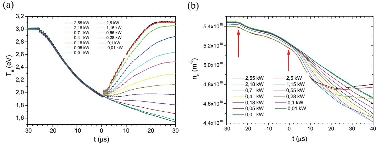
Fig.4: Evolution of the electron temperature (a) and density (b) during the double  $rf$  pulse for different  $rf$  powers (pause 22  $\mu\text{s}$ ,  $B = 40.5$  mT,  $P_{Ar} = 0.3$  Pa,  $P = 1.4$  kW,  $z = 25$  cm).
