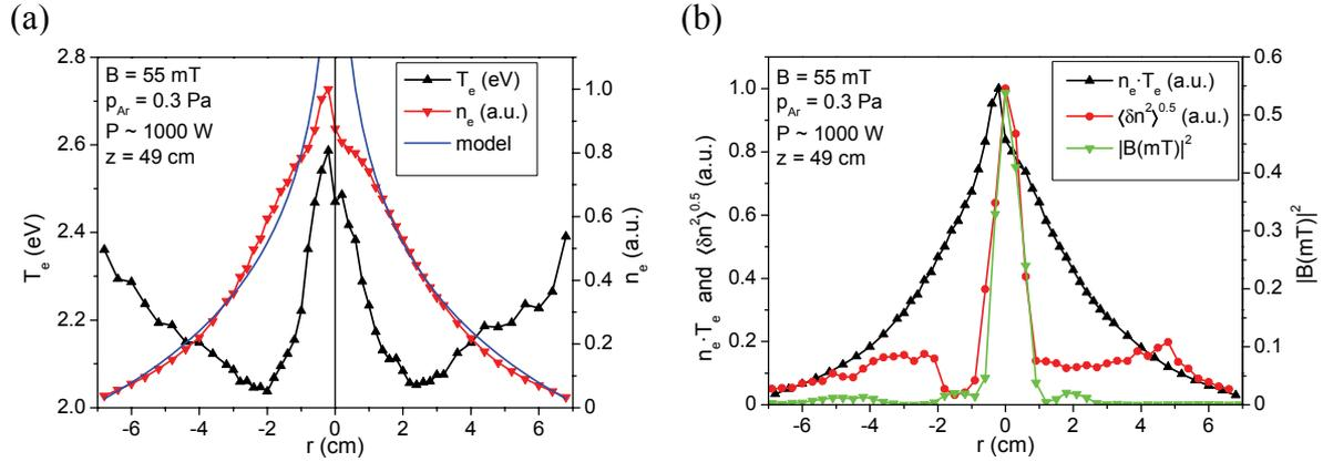
Fig3: Profiles of electron density and temperature (a) and thermal energy density, magnetic energy density and fluctuation amplitude (b) 49 cm away from centre of antenna.
