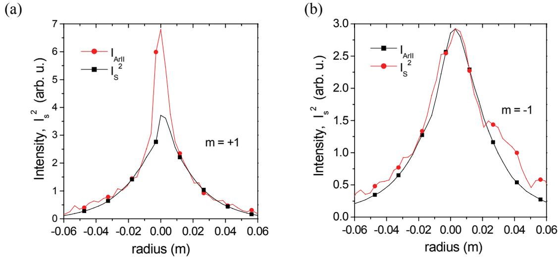
Fig2: Radial profile of the 480.6 nm argon ion emission and the squared ion saturation current 25 cm away from the centre of the antenna for the  $m = +1$  (a) and  $m = -1$  side (b) ( $B = 54$  mT,  $P = 0.2$  Pa,  $P = 1.4$  kW).
