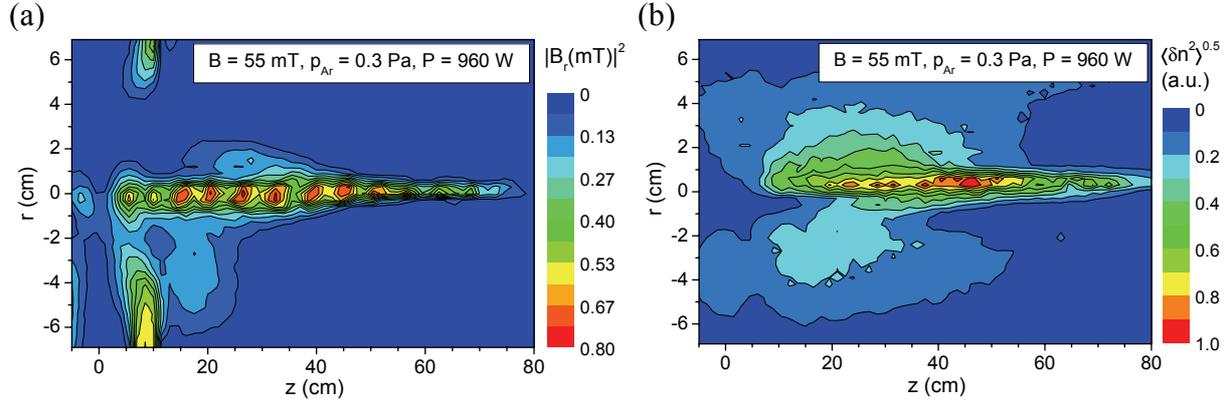
Fig1: Contour plots of the  $rf$  magnetic field energy (a) and density fluctuation amplitude (b) for the  $m = +1$  side (centre of antenna at  $r = z = 0$ ).
