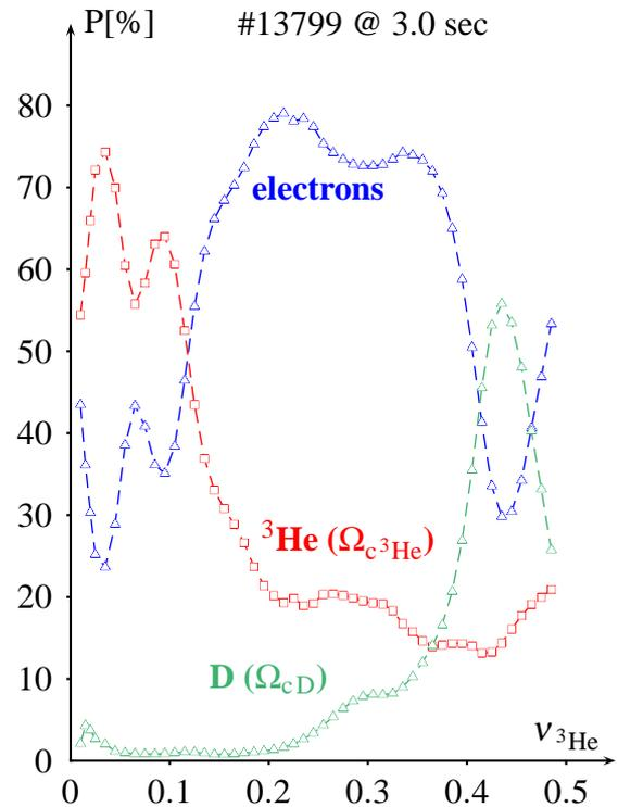
Figure 2: rf power distribution in a D(<sup>3</sup>He) plasma as function of <sup>3</sup>He concentration.
