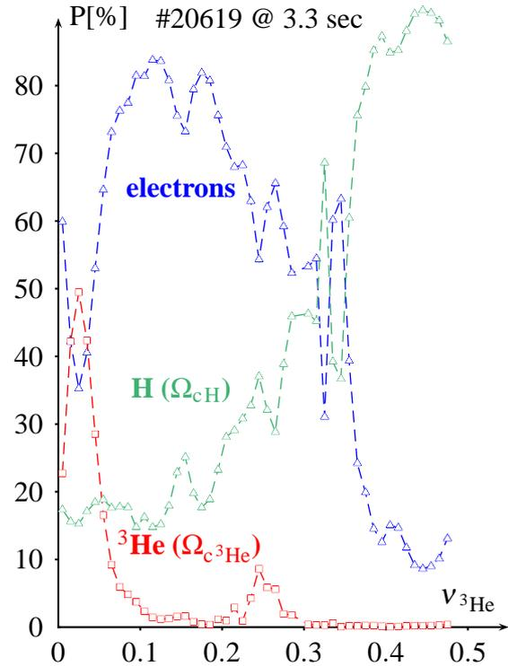
Figure 3: rf power distribution in a  $\text{H}(^3\text{He})$  plasma as function of  $^3\text{He}$  concentration.
