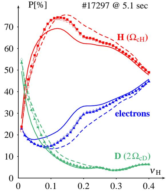
Figure 1: rf power distribution in a D(H) plasma as function of the H concentration for  $n_\phi = 12$ : solid lines with Maxwellian distribution functions (df) for the minority, open symbols with df calculated by SSFPQL with 4 MW of coupled power, and full symbols are the second iteration of TORIC-SSFPQL. The dashed lines are the first iteration with 10 MW of rf power.
