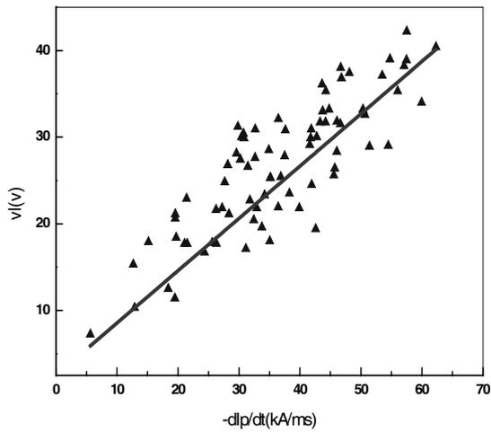
Fig.3 The current average decay rates versus the maximal loop voltage during disruption. The triangle symbol stands for the experimental data and the line stands for the simulation results
