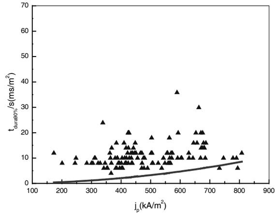
Fig.2 Time average current quench times divided by plasma cross-section area versus plasma current density before disruption
