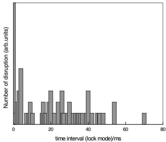
Fig.4 The relation between time interval and number of disruption
