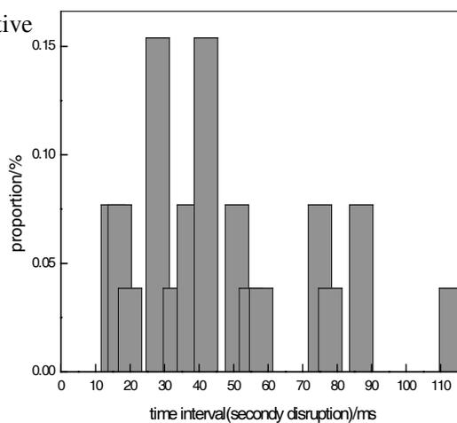
Fig.5 The relation between time interval and disruption proportion
