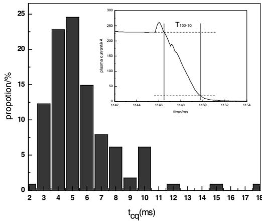
Fig.1 Histogram of current quench time obtained from 100-10% current thresholds in HL-2A
