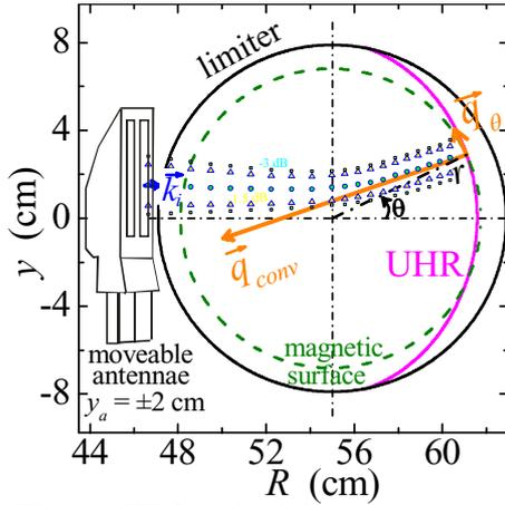
Fig. 1. FT-2 poloidal cross section ( $\vec{k}_i$  – incident wave vector,  $\vec{q}_{conv}$  and  $\vec{q}_\theta$  – fluctuation wave vector at BS efficiency maximum and it's poloidal projection, circles – central ray of the probing beam, triangles and squares – probing beam at 1.5 and 3 dB power suppression levels).
