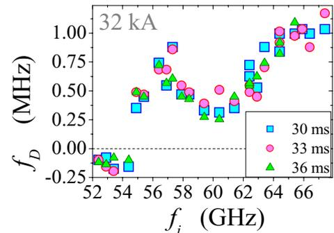
Fig. 2. The UHR BS Doppler frequency shift versus probing frequency.
