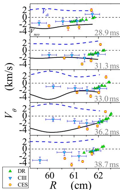
Fig. 5. Poloidal velocity profiles in current ramp up experiment.
