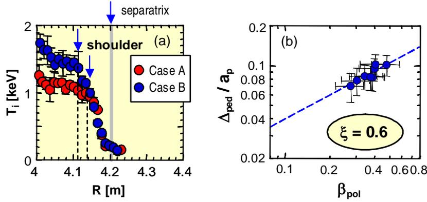
**Figure 6.** (a) Pedestal  $T_i$  profiles for the  $\beta_{pol}$  scan at the same  $\rho_{pol}^*$  and  $v^*$ . (b) Relation between  $\beta_{pol}$  and  $\Delta_{ped}/a_p$  at  $\rho_{pol}^* \sim 4.5 \times 10^{-2}$ . The exponent of  $\beta_{pol}$  in the log-linear regression at fixed  $\rho_{pol}^*$  is  $\xi = 0.6$ .
