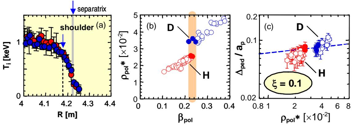
**Figure 4.** (a) Pedestal  $T_i$  profiles for deuterium and hydrogen plasmas at the same  $\beta_{pol}$  and  $v^*$ . (b) Data area in  $\beta_{pol}$ - $\rho_{pol}^*$  space of the experiments. (c) Relation between  $\rho_{pol}^*$  and  $\Delta_{ped}/a_p$ . The exponent of  $\rho_{pol}^*$  in the log-linear regression at fixed  $\beta_{pol}$  is  $\xi = 0.1$ .
