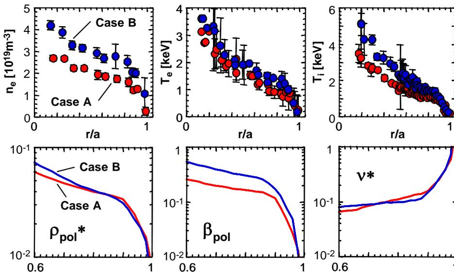
**Figure 5.** Profiles of  $n_e$ ,  $T_e$ ,  $T_i$  for  $\beta_{pol}$  scan experiments. Edge profiles of  $\rho_{pol}^*$ ,  $\beta_{pol}$  and  $v^*$  are also shown.
