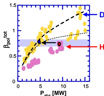
Figure 1. Relation between  $P_{\text{abs}}$  and  $\beta_{\text{pol}}^{\text{tot}}$  for hydrogen and deuterium discharges.
