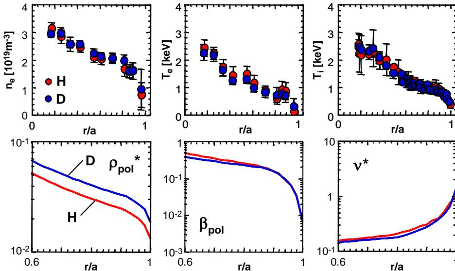
**Figure 3.** Profiles of  $n_e$ ,  $T_e$ ,  $T_i$  for deuterium and hydrogen discharges. Edge profiles of  $\rho_{\text{pol}}^*$ ,  $\beta_{\text{pol}}$  and  $v^*$  are also shown.
