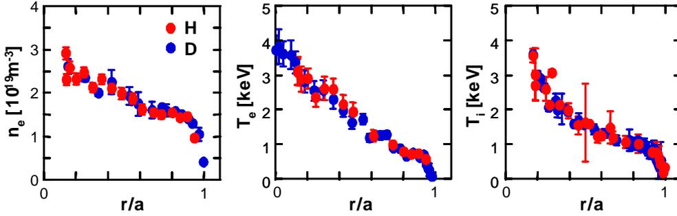
**Figure 2.** Profiles of  $n_e$ ,  $T_e$  and  $T_i$  which correspond to the deuterium and hydrogen discharges operated at the same  $\beta_{\text{pol}}^{\text{tot}}$  (see highlighted data points shown in figure 1).
