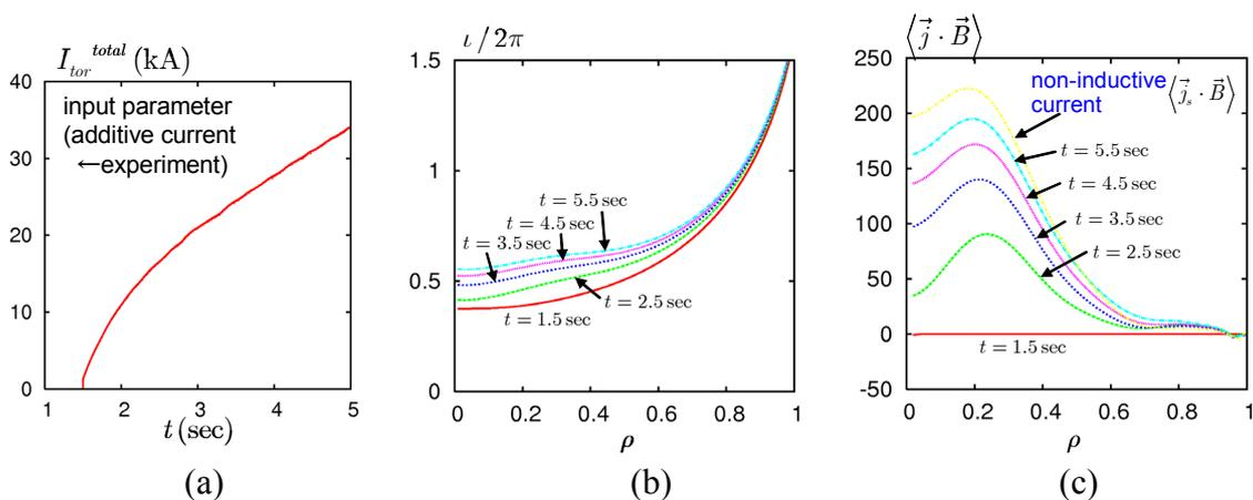
Fig.4 The results of time evolution simulation of the rotational transform and the net current in the presence of the non-inductive current in an LHD plasma: (a) time history of specified total toroidal current which is measured in the experiment, (b) time evolution of the rotational transform profile, and (c) time evolution of the net parallel current density profile.
