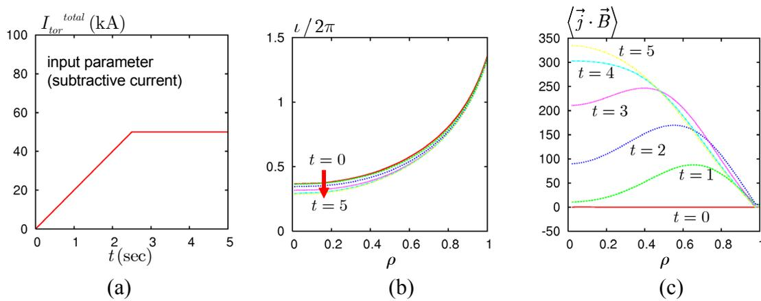
Fig. 3 Current ramp-up simulation: (a) time history of specified total toroidal current, (b) time evolution of rotational transform profile, and (c) time evolution of parallel current density profile.
