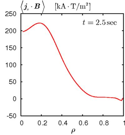
Fig.2 The non-inductive current at  $t = 2.5s$  calculated by the BSC/FIT code.
