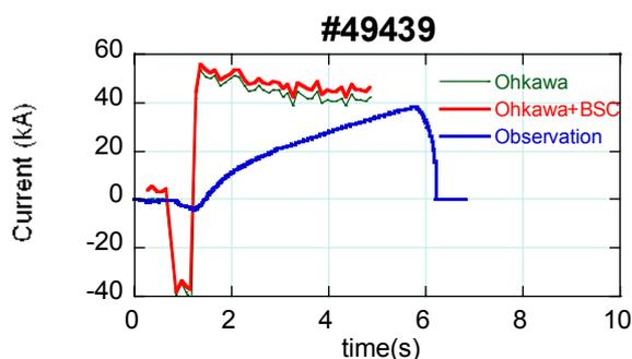
Fig.1 Time evolution of net toroidal currents in a LHD discharge with 2 NB injections.
