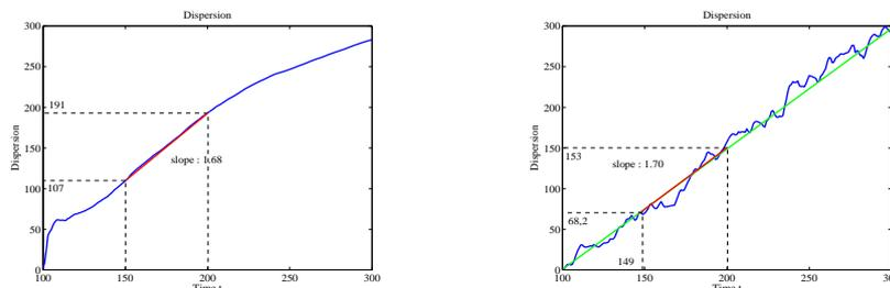
(a) Diffusion of impurity as fluid (b) Diffusion of impurity as particle
