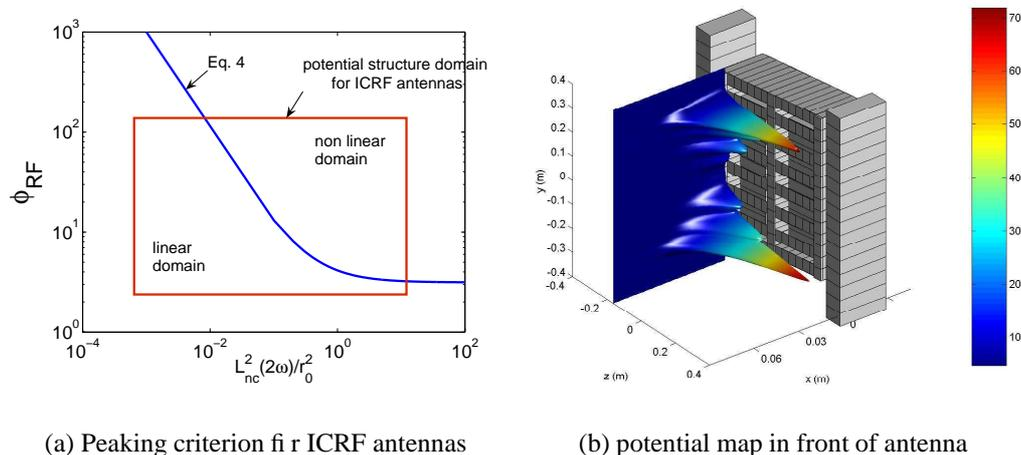
Figure 4: (a) : Peaking criterion at the summit of the Gaussian potential at different frequencies. (b) : 2D DC potential map obtained in a poloidal plane in front of an ICRF antenna composed of a simplified Faraday screen.
