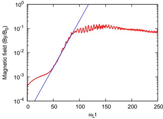
Figure 3. Temporal profile of the self-generated magnetic field  $B_y / B_0$  at logscale.
