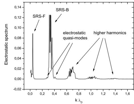
Figure 1: A fully developed electrostatic k-spectrum in the non-linear stage of SRS with the spectral broadened peak of SRS-B due to the present TPI. A shift of the central EPW belonging to SRS-B towards the lower side-band is clearly seen.
